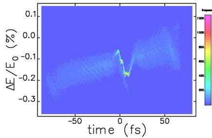
Figure 2: Longitudinal phase space at the exit of the linac.
