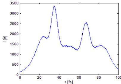
Figure 6: Electron beam current profile for the under-compression case with double-slot foil (bunch head is to the right).
