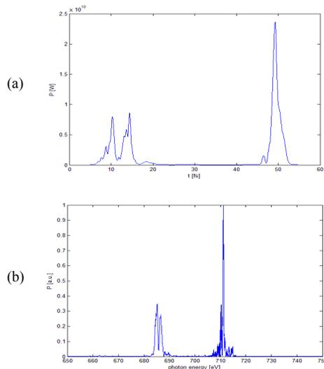
Figure 3: Output radiation pulses (a) and corresponding spectrum (b) generated by the first scheme.
