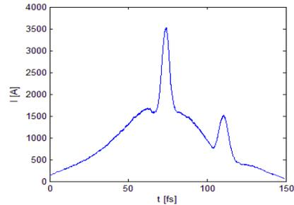
Figure 4: Electron beam current profile for the over-compression case with double-slot foil (bunch head is to the right).
