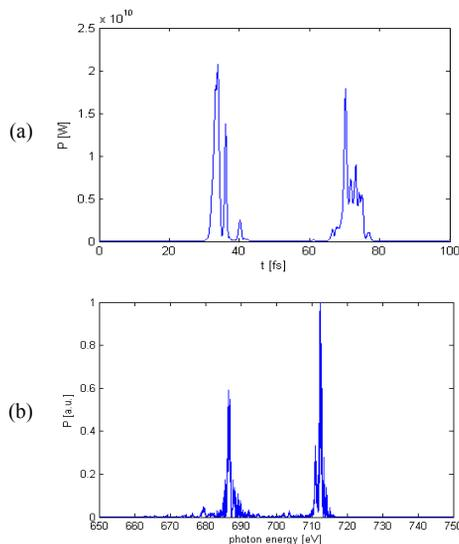
Figure 7: Output radiation pulses (a) and corresponding spectrum (b) generated by the second scheme.
