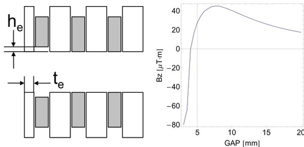
Figure 3: On the left, the schematic of the end design, where the height of the first (last) pole and the thickness of the first (last) magnet are used to march the trajectory. On the right, the kick experienced by the electron both at the entrance and at the exit of the undulator, only for one gap the match can be achieved.
