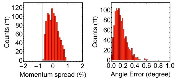
Figure 1: The statistics of the first 1400 magnets produced by Hitachi. On the left the momentum spread and on the right the magnetization angle error.
