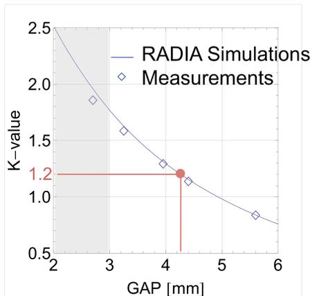
Figure 6: The K-value versus gap calculated with the computer code RADIA versus the magnetic measurements on the short prototype
