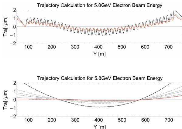
Figure 7: The horizontal (top) and vertical (bottom) trajectories calculated at 5.8 GeV before the optimization.
