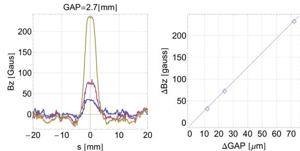
Figure 8: On the left the field profile change due to three different local gap changes, on the right their amplitude as a function of the actual gap variation.
