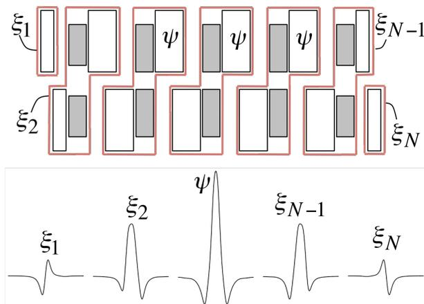
Figure 9: On the top the schematic representation of the undulator poles (grey) and magnets (white) as they are grouped in terms of local gap changes. On the bottom the impact of the local gap change on the magnetic field for the different groups.
