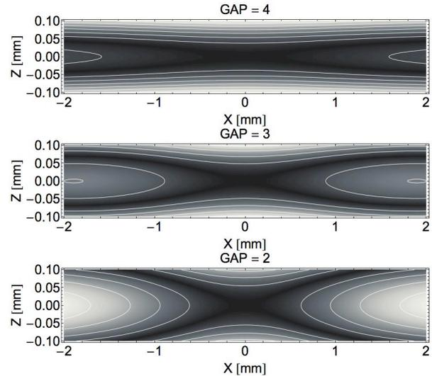
Figure 4: The field homogeneity in a U15 cross section is calculated with RADIA for different gaps. The inner most line represent relative deviation with respect to the central field of  $10^{-4}$ , the second is  $2 \cdot 10^{-4}$  and so on.
