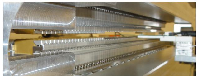
Figure 5: The short prototype undulator side view during the magnetic measurements. On the right side the hall probe head driven by a granite bench.
