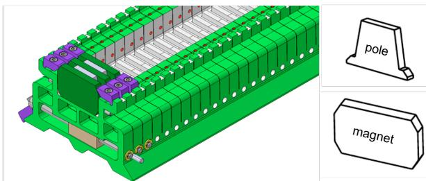
Figure 2: The aluminium extruded block keeper, design to hold 22 periods.
