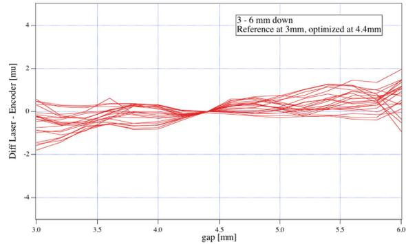
Figure 7: Gap variation versus Heidenhain encoder settings for gaps between 3 and 6mm in 0.2mm steps. The curves are referenced to a gap of 4.4mm (nominal K-value of 1.2) where the U15's will be optimized.
