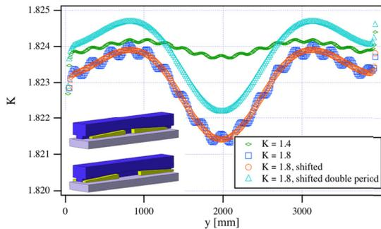
Figure 3: Simulated K-variation with gap change based on FEM and RADIA calculations. At K=1.2 (gap=4.4mm) the ID will be optimized, the different forces at K=1.4(1.8), gap=3.8(3)mm, lead to deformations in the outer and inner I-beam (long range and short range variations). A shifted arrangement of the columns (see next section) flattens the high frequency oscillations, even with reduced number of columns. The sketch shows the wedge settings for open (top) and closed gap (bottom).
