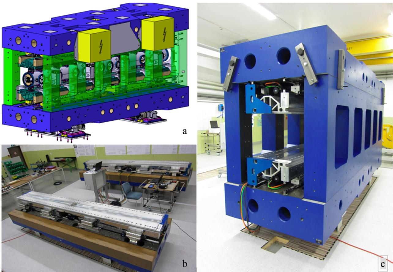
Figure 1: U15 in-vacuum prototype undulator: a) 3D CATIA sketch, b) assembling of top and bottom bases, c) completed support structure before the final gluing of the top bases with the side parts at MDC Max Daetwyler Corporation in Ursenbach, Switzerland.
