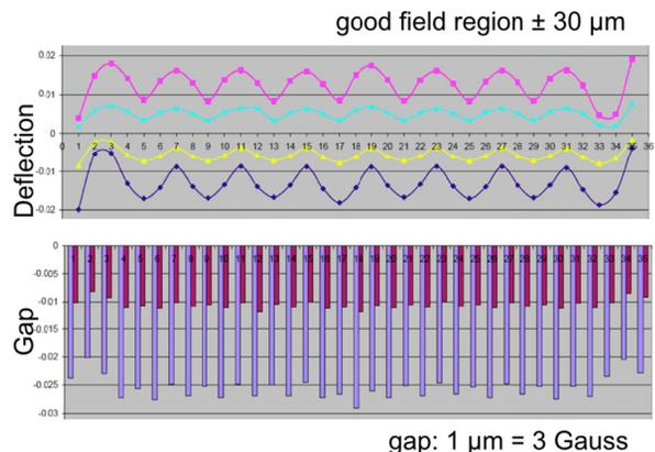
Figure 5: FEM calculations of deflections of top and bottom I-beam and resulting gap variation which is constant within 1μm for K=1.4 and 2μm for K=1.8.
