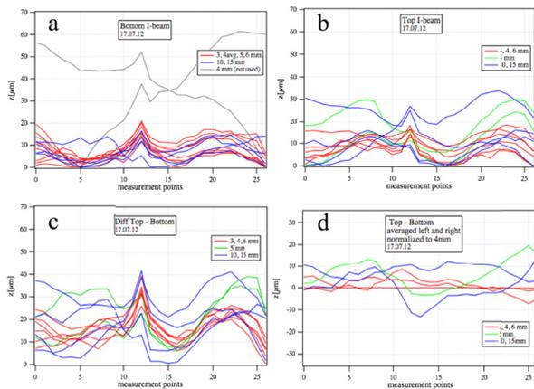
Figure 6: Flatness and calculated gap versus the longitudinal position of the outer I-beams (a,b), measured with the Wyler electronic inclinometer. The measurements show clearly the areas without direct support of the wedge bearing system. The variation with gap (d) is the remaining error.
