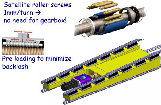
Figure 2: SwissFEL undulator drive system with servo motor, satellite roller screw and wedge sandwiched by bearings.
