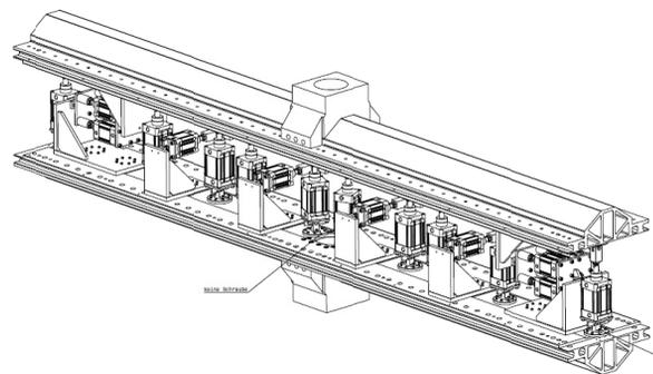
Figure 8: Pneumatic cylinder to simulate forces up to 3 tons in planar and APPLE II configuration.
