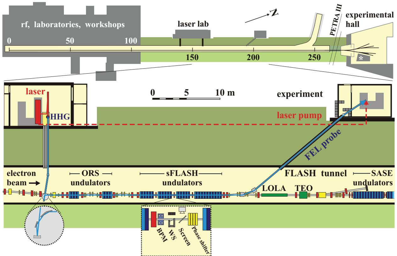
Figure 1: Schematic of the sFLASH experiment as part of the FLASH facility. FLASH (top part) has an overall tunnel length of 260 m, out of which 40 m are dedicated to the XUV seeding experiment (bottom part). Indicated components are dipole magnets (yellow), quadrupole magnets (red), undulator magnets (blue).
