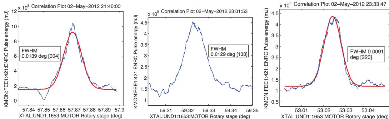
Figure 6: Intensity after the Kmono as a function of the seeding crystal angle for three different crystal planes.
