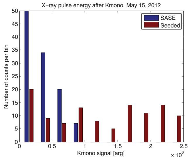
Figure 3: Histograms of intensity after the Kmono for tuned-up SASE operation and for a seeded beam.
