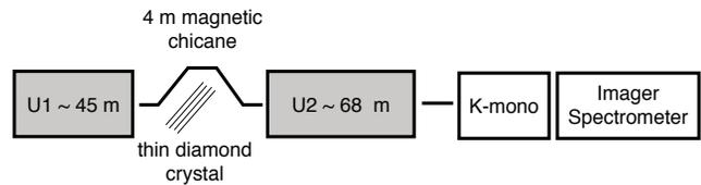
Figure 1: Schematic of hard x-ray seeding at LCLS.
