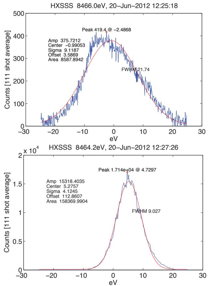
Figure 5: Average SASE spectrum at the seeding chicane (top) and at the output of LCLS (bottom) for normal SASE operation.
