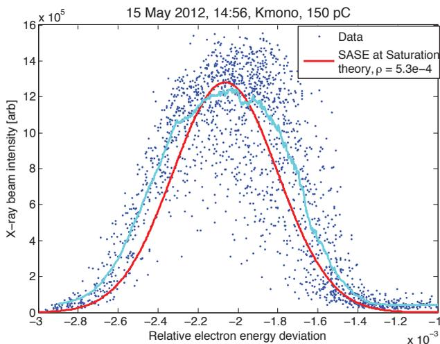
Figure 4: Correlation of electron energy with the x-ray intensity (pulse energy) after passing the seeded beam through the Kmono. The cyan curve is a running average while the red curve is a theoretical curve shown for reference.
