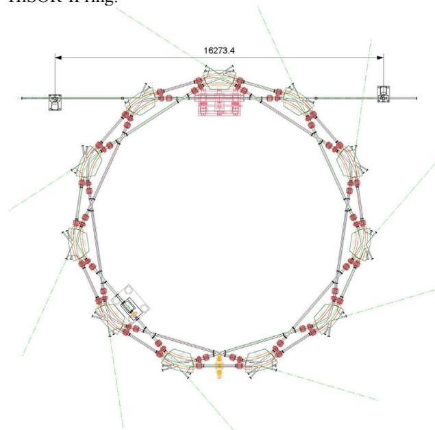
Figure 6: Oscillator FEL configuration in HiSOR-II ring.
