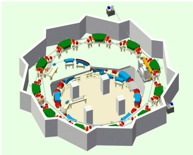
Figure 7: Designer's view of HiSOR-II ring with an oscillator FEL section.
