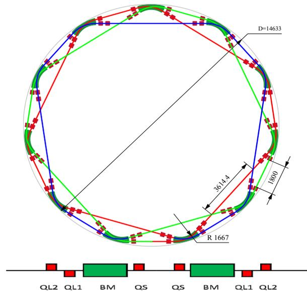
Figure 4: An example of (11,3) torus knot lattice for a compact light source and a unit cell.
