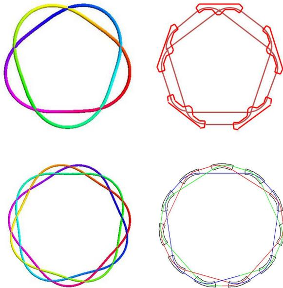
Figure 3: Examples of projected torus knots and bending magnet configurations of corresponding lattices.
