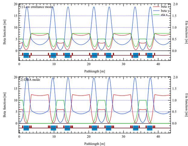
Figure 5: Optical functions on each operating point. 1):Low emittance mode, 2):DBA mode.
