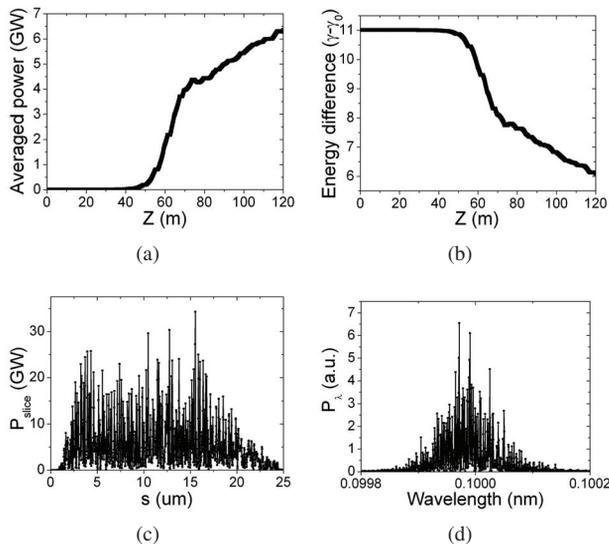
Figure 4: An example of time-dependent simulation. (a) radiation power is saturated at 75m and slowly growing, (b) averaged energy is reduced with lasing, (c) peak power reaches 30GW while averaged power is 4.5GW at 75m and (d) radiation wavelength is centered at 0.1nm with  $3 \times 10^{-4}$  width.
