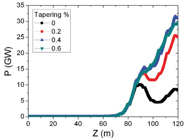
Figure 5: Tapering in steady-state simulation.
