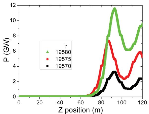
Figure 2: SASE lasing in steady-state with various energy.
