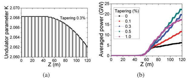
Figure 6: Tapering in time-dependent simulation. (a) 0.3-0.5% quadratic tapering is effective. (b) Variation of undulator parameter in case of 0.3% tapering.
