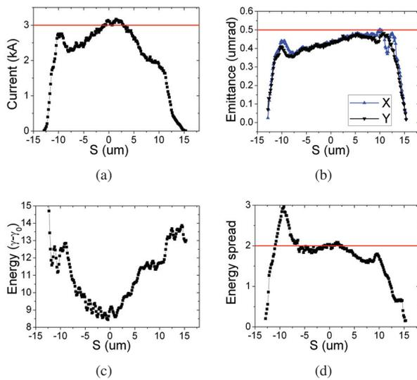
Figure 3: Slice properties of input beamfile for time-dependent simulation. (a) Beam current is smaller than target value, (b) normalized transverse emittances are slightly lower than requirements, (c) energy is selected by scan-test and (d) energy spread is acceptable.
