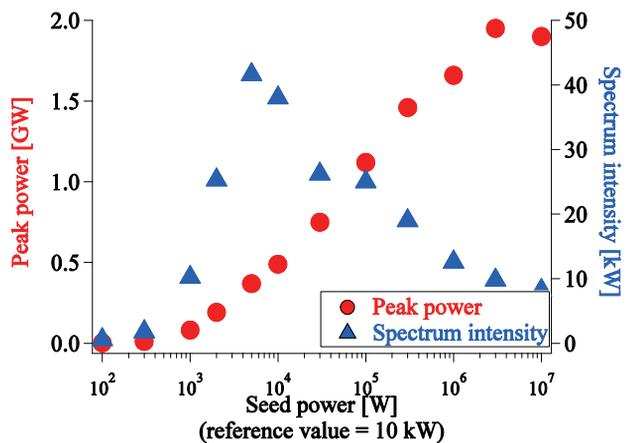
Figure 8: Power dependences on the seed power without changing of the seed pulse duration in the 20 nm cascaded FEL case.
