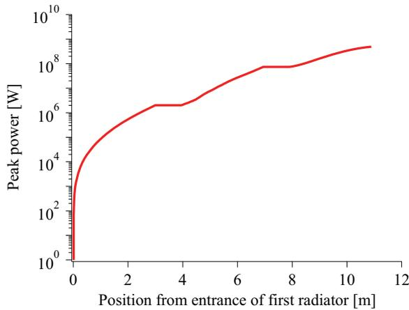
Figure 2: FEL peak power evolution calculated by GENESIS in the 20 nm cascaded FEL case.
