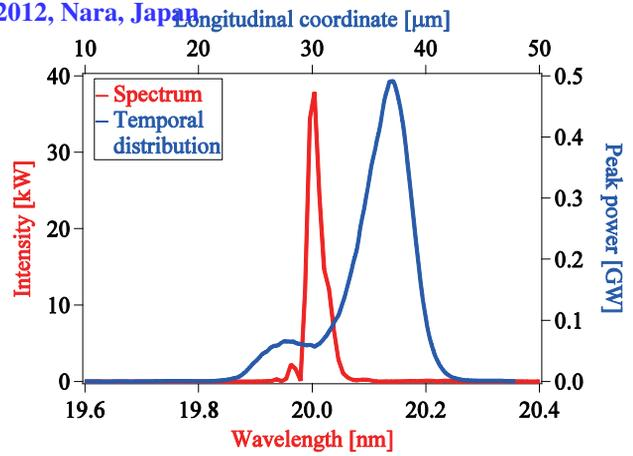
Figure 3: Spectral (red solid line) and temporal (blue solid line) distributions calculated by GENESIS in the 20 nm cascaded FEL case.
