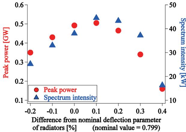
Figure 9: Power dependences on the deflection parameter of the radiators in the 20 nm cascaded FEL case.
