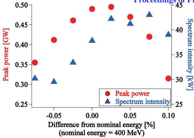
Figure 4: Power dependences on the beam energy in the 20 nm cascaded FEL case.
