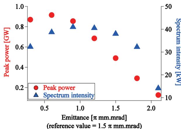
Figure 6: Power dependences on the beam emittance in the 20 nm cascaded FEL case. The matching condition at the undulators isn't changed from the reference case.
