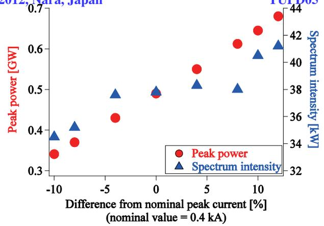
Figure 7: Power dependences on the peak current without changing of the bunch length in the 20 nm cascaded FEL case.
