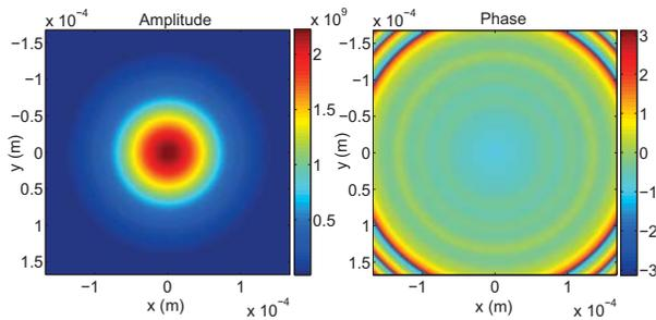
Figure 3: Amplitude and phase of the sixth harmonic at the maximum of the intensity.
