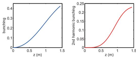
Figure 4: Bunching at the fundamental wavelength and its second harmonic along the modulator.
