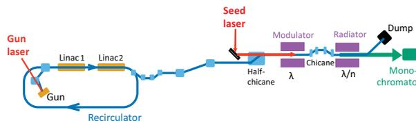
Figure 1: Layout of the experimental setup.
