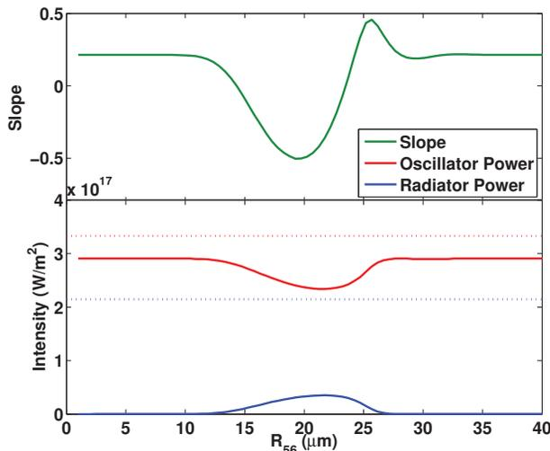
Figure 2: Bottom plot: Equilibrium intensity of oscillator (red) and radiator (blue); dashed lines show nominal saturation values. Top plot: Slope of transfer map from one pass to the next; values with magnitude  $> 1$  would correspond to unstable dynamics, leading to oscillations.
