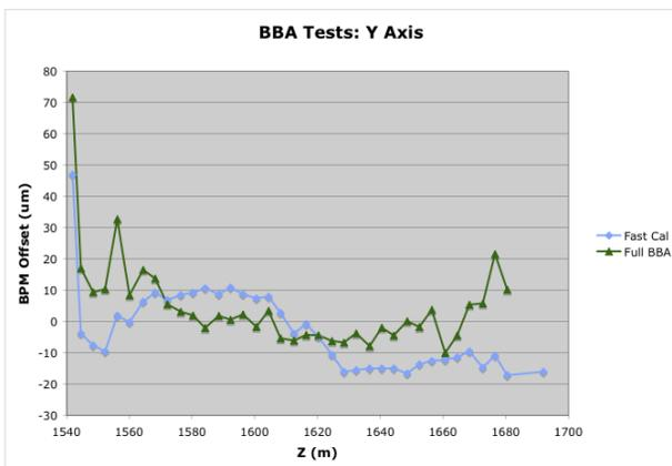
Figure 6: BPM offset corrections for Y axis from Fast Cal and Full BBA (August 5, 2012).
