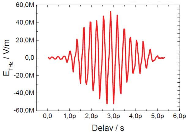
Figure 2: 3 THz pulse of the pilot super-radiant THz facility at FLASH [5] sampled via photoelectron streaking by naturally synchronized fs X-ray pulses[8],[10]. For a sub-cycle sampling at 3 THz a sub 100 fs synchronization is required.
