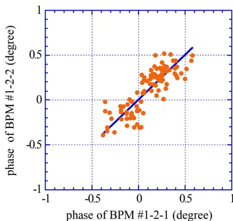
Figure 2: A correlation plot of the measured phases from two adjacent BPMs.
