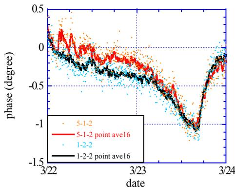
Figure 5: The BPM phases measured at an entrance (#1-2-2) and an exit (#5-1-2) of the BL3 undulator section for two days.
