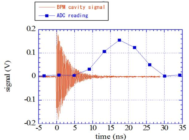
Figure 3: A waveform from a BPM reference cavity and an output signal from an IQ demodulator. The beam charge was 0.2 nC.
