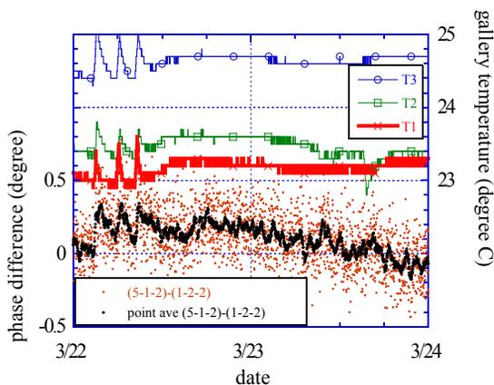
Figure 6: The trend of the phase difference of two BPMs at the BL3 undulator section (red and black dots). Some of the ambient temperatures in the undulator gallery where the optical cable and the 19” racks are located are also shown (solid lines).
