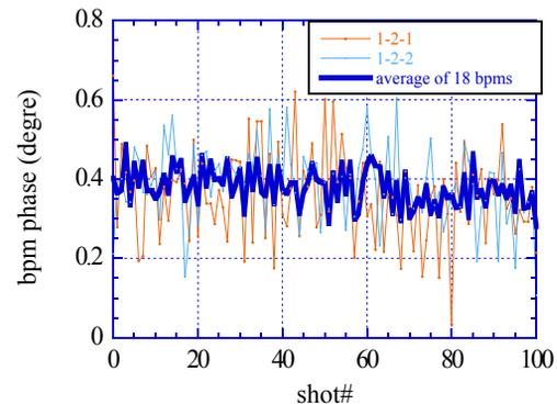
Figure 4: The trend of the beam phases of the two BPMs for 10 second measurement. The averaged phase of the eighteen BPMs located at the BL3 undulator is also shown.
