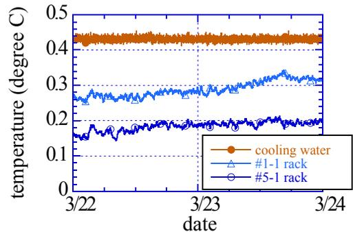
Figure 7: A temperature of the cooling water of the undulator section and 19” racks of #1-1 and #5-1 BPMs.
