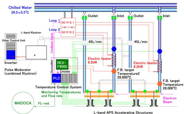
Figure 4: Schematic drawing of the precise temperature-regulation system for one L-band accelerating unit.
