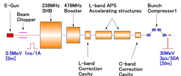
Figure 1: Schematic layout of an injector at SACLA.
