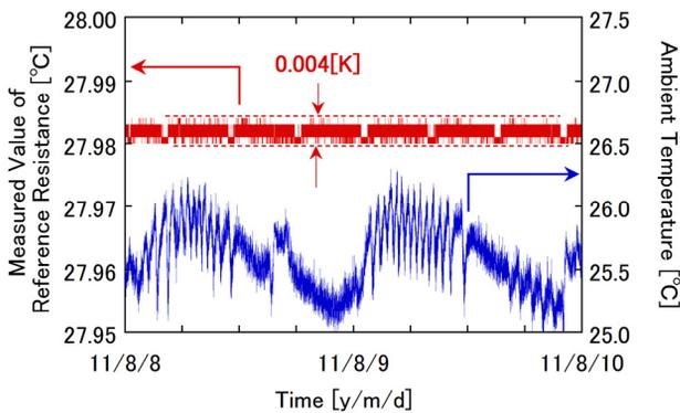
Figure 3: Trend graphs of measured values by using a new temperature measurement and control module with a high precise reference resistance (red) and the ambient temperature (blue).
