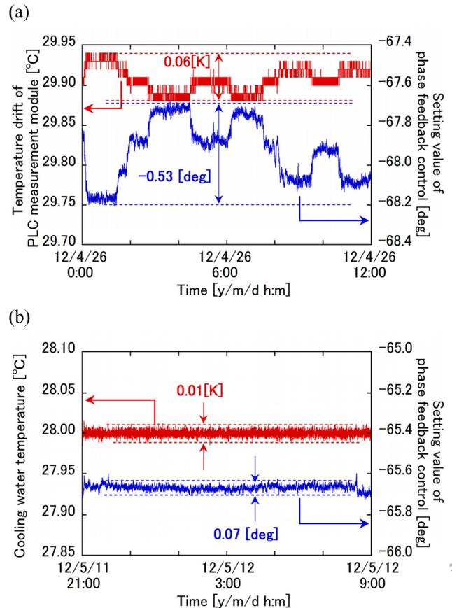
Figure 5: Comparison of the temperature regulation performance between feedback control with the PLC and that with REX-F9000. (a) Trend graphs of temperature drift (red) and a setting value of phase feedback control (blue) for 238MHz SHB. (Feedback control with the PLC). (b) Trend graphs of cooling water temperature (red) and a setting value of phase feedback control (blue) for 238MHz SHB. (Feedback control with REX-F9000).
