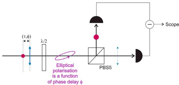
Figure 2: Phase delay monitor using polarisation interference. The pulses interfere to give a total elliptical polarisation which has ellipticity as a function of  $\phi$ . The visibility of the fringes is a function of  $\tau$ .
