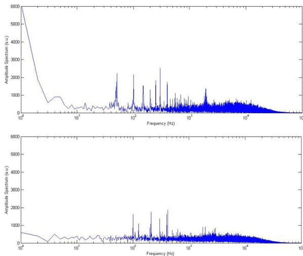
Figure 5: Spectrum of fringes when the link is unlocked (top) and locked (bottom).
