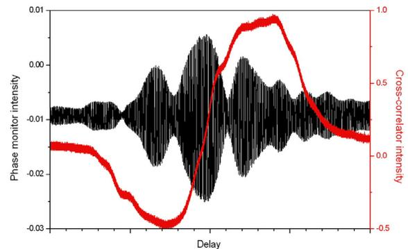
Figure 3: Relative positions of phase (black) and group (red) monitor signals over an approx. 2ps range.
