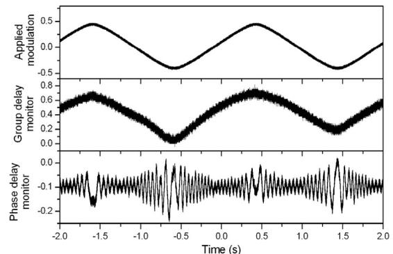
Figure 4: Phase and group monitoring of a 0.5 Hz modulation applied to the fibre stretcher.
