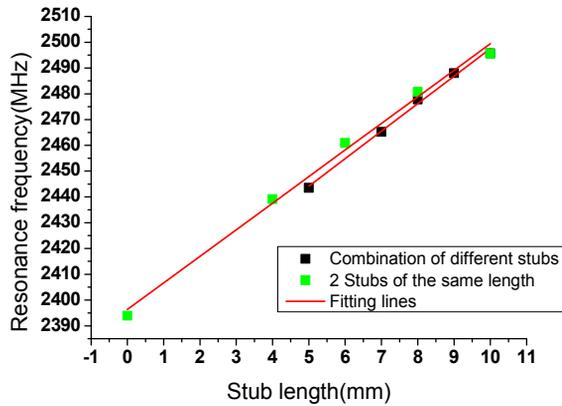
Figure 7: Variation of stubs with different length as compared with stubs of same length.
