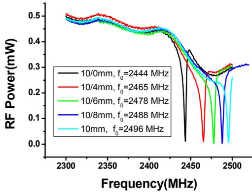
Figure 6: Resonance tuning by combination of stubs with different length.
