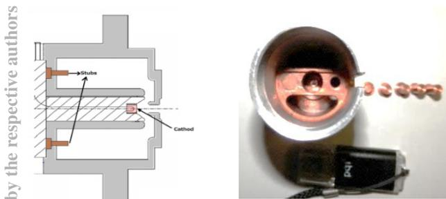
Figure 4: Stub tuning system of the coaxial triode cavity.
