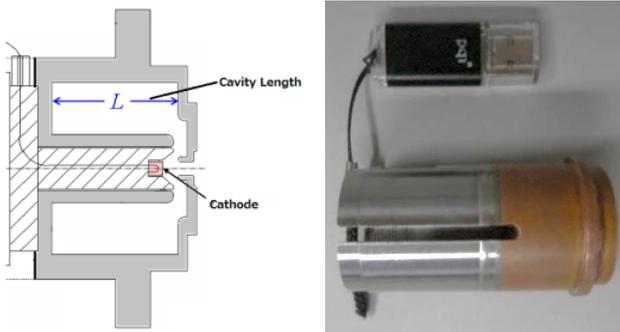
Figure 2: Schematic cross-section of the triode cavity and side view of fabricated prototype.
