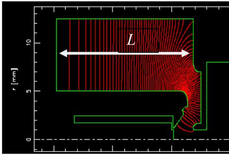
(a) Simulation of ele. Field distribution in cross section of cavity according to old design
