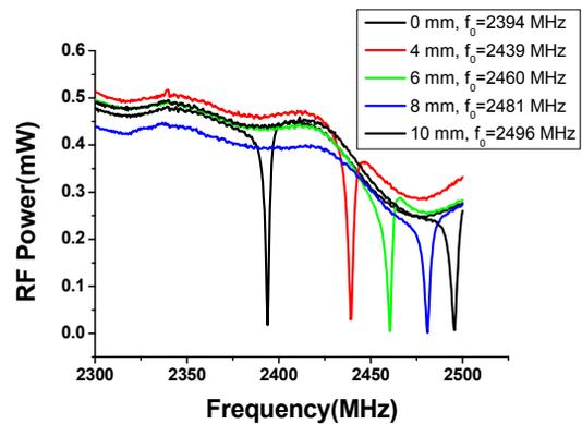
Figure 5: Measured dependency of resonance frequency on stub length.
