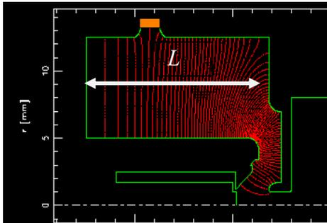
(b) Simulation of ele. Field distribution in cross section of cavity according to new design
