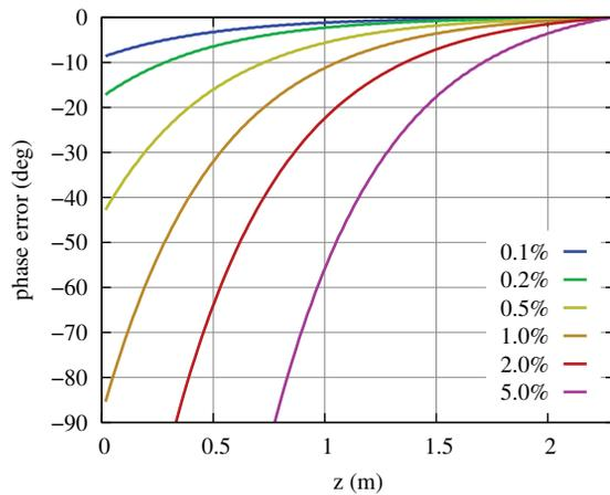
Figure 2: Phase errors for various demagnetization profiles.
