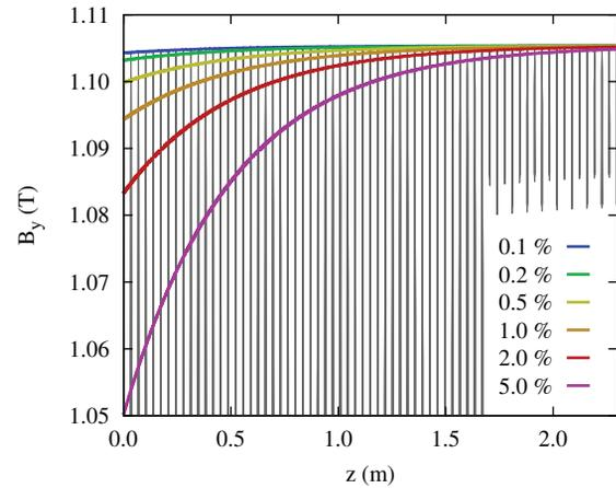
Figure 1: Undulator magnetic field profiles for phase error calculations. Colored lines indicate the tapered field amplitudes, gray lines show the actual oscillating magnetic field.
