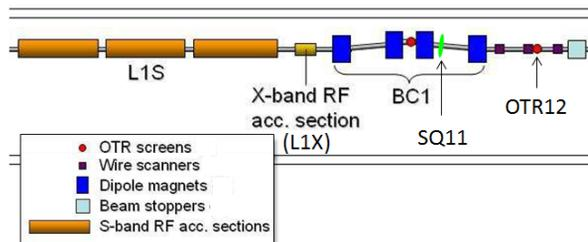
Figure 1: Layout of *LCLS* injector in the BC1 area. The 9-m long S-band linac section (L1S) is followed by a 60-cm long X-band RF section (L1X) feeding the BC1 chicane at 220 MeV. The “SQ11” skew quad and “OTR12” screen are also shown.
