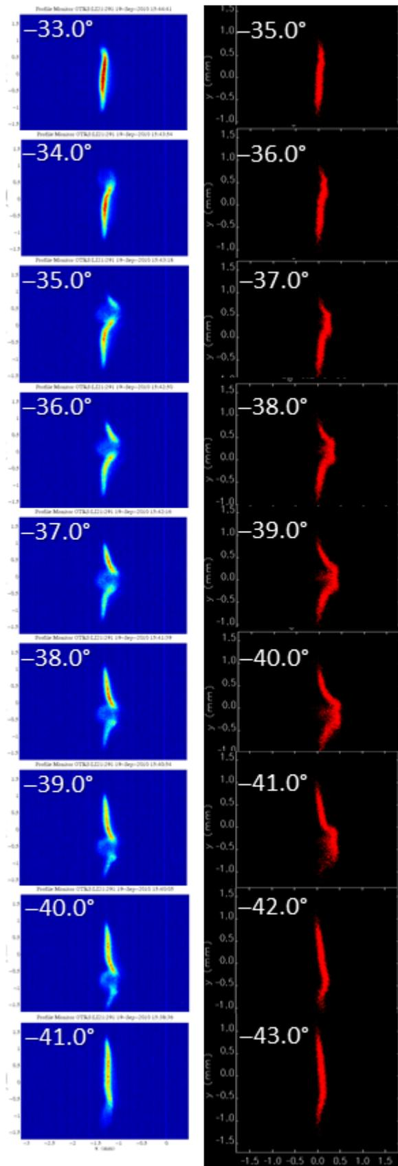
Figure 6: Measurements (left) and simulations (right) with X-band RF switched off. The LIS phase settings differ between measurement and simulation by  $2^\circ$ .
