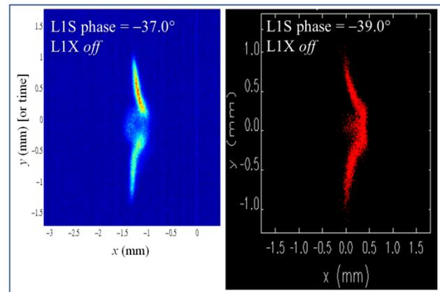
Figure 5: Measured image (left, at  $-37^\circ$ ) and simulated (right, at  $-39^\circ$ ) with L1X RF switched off. The L1S phase differs between measurement and simulation by  $2^\circ$ .
