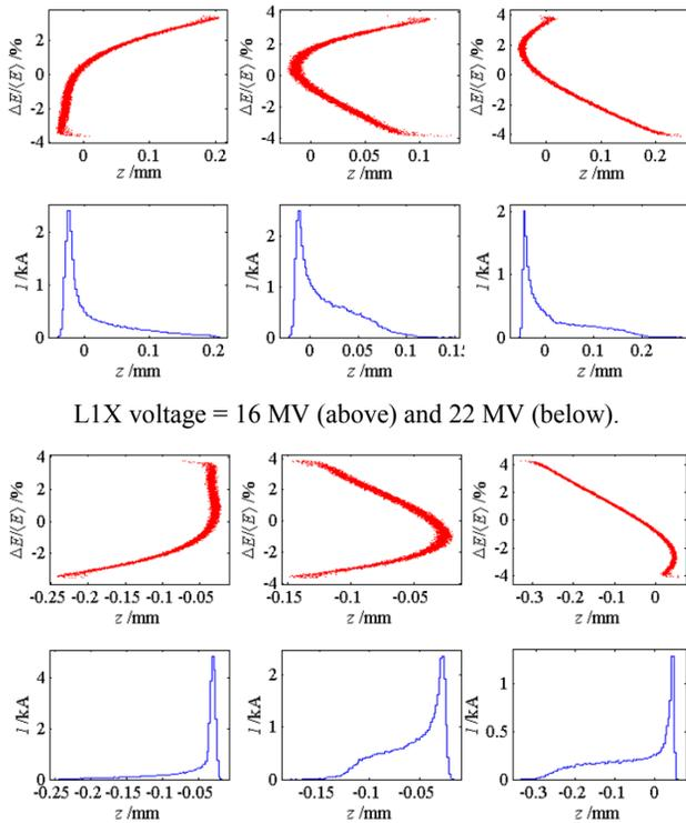
Figure 3: Simulation explaining evolving images in Figure 2 with two L1X voltage settings (top six plots at 16 MV and bottom six at 22 MV). Each of the three columns are for different L1S phases. Parameters are approximate here simply to help explain the effect.
