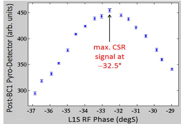
Figure 4: Post-BC1 pyroelectric CSR detector reading vs. L1S RF phase at  $V_{L1X} = 16$  MV with maximum at  $-32.5^\circ$ .
