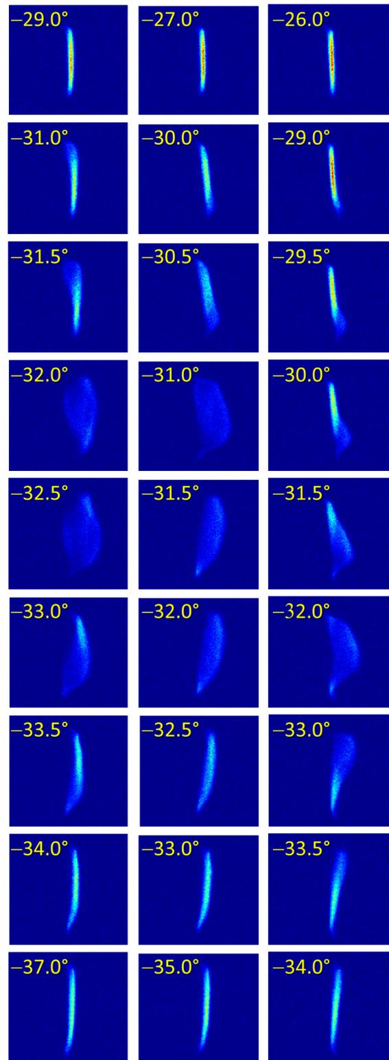
Figure 2: OTR screen images with the X-band RF set at 16 MV (left column), 19 MV (center), and 22 MV (right). The bunch length (vertical streak) here is  $\sim 6$  ps FWHM with the pre-BC1 bunch *head* at the top of each image. Energy loss in the final BC1 bend kicks to the right here.
