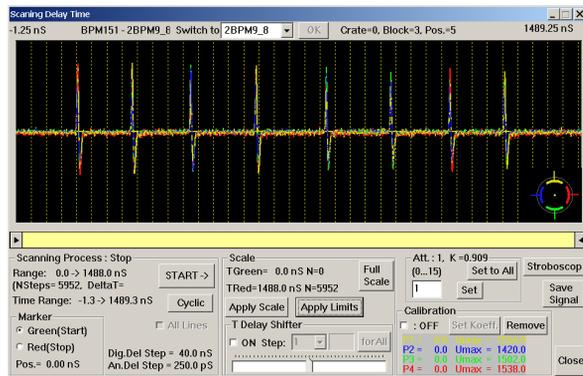
Figure 7: Signal from the BPM installed near the dump.
