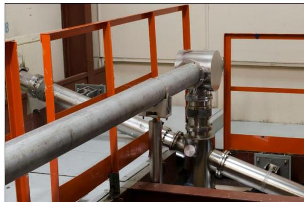
Figure 5: Optical beamlines for the first and the second stage FELs. Radiation of both FELs is delivered to the same user stations. Switching between FELs is done by retractable mirror.
