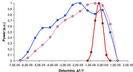
Figure 4: Normalized detuning curves for the lasing at the first (blue) and third (red) harmonics and the detuning curve for the amplified spontaneous emission at the third harmonic (pink).
