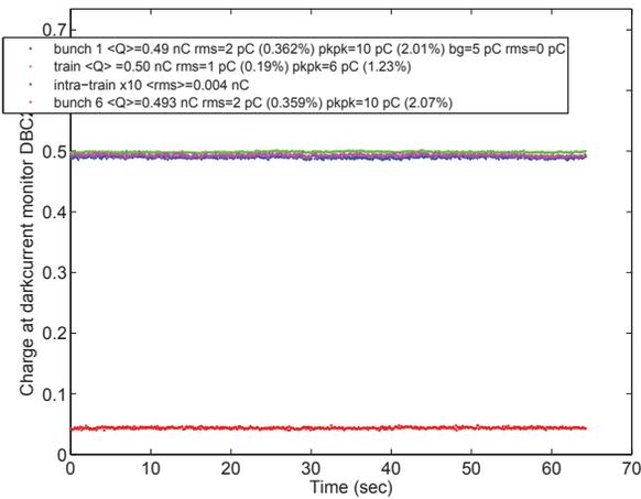
Figure 4: Measured charge in the FLASH accelerator. Shown is the charge of bunches 1 and 6 (blue, magenta) and also averaged over the train (green). The intra train rms jitter is shown in red with a magnification of 10. The rms stability of a single bunch from shot to shot is 0.36 %, and average over the pulse train, 0.19 %. In this example, 1250 bunches per second have been accelerated.
