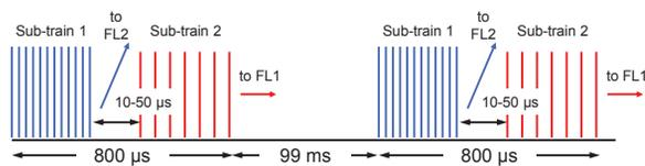
Figure 5: Bunch train sharing between FLASH1 (FL1) and FLASH2 (FL2): one RF pulse is shared by two sub-bunch trains. One train goes to FLASH1, the other is kicked to FLASH2. The sub-trains may have different bunch pattern or energy as indicated.
