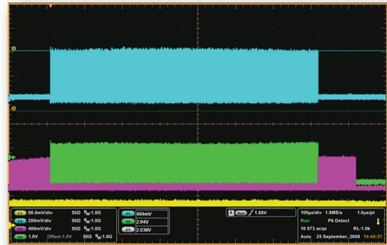
Figure 2: Example of a 3 MHz laser pulse train. The oscilloscope traces show the pulse train of the oscillator (yellow trace), after preamplification (wavelength 1047 nm, magenta), after conversion to 523 nm (green), and after conversion to the UV (262 nm, blue). The time scale is 1 ms (whole range). The train length is 700  $\mu$ s. The 3 MHz pulse structure is not resolved.
