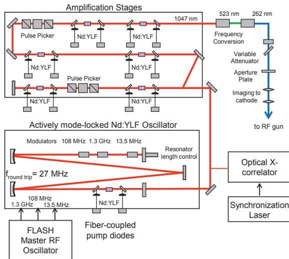
Figure 1: Schematic overview of the laser system. The second new laser has a more modern shorter oscillator operated at 108 MHz.
