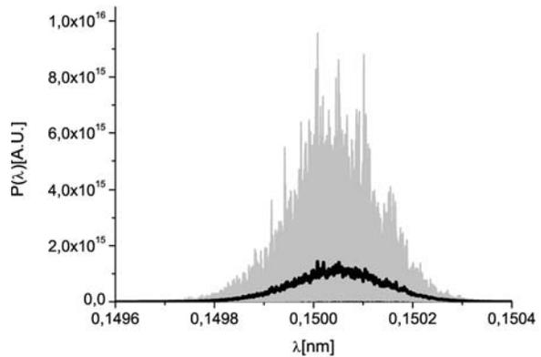
Figure 9: Upper plot: SASE power at the exit of the first 10 FEL undulator cells. Lower plot: SASE spectrum at the exit of the first 10 FEL undulator cells.
