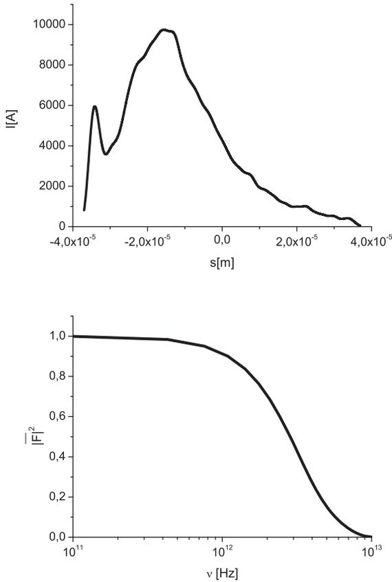
Figure 5: Upper plot: Electron beam current profile at the European XFEL, optimized for THz pump/X-ray probe experiments. Lower plot: Squared modulus of the electron beam form factor,  $|\bar{F}|^2$ , corresponding to the current profile on the upper plot.
