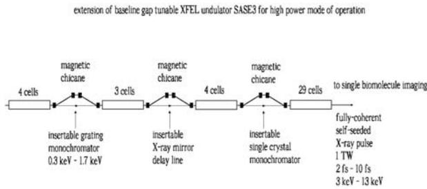
Figure 1: Design of the undulator system for the bio-imaging beamline. The method exploits a combination of self-seeding, fresh bunch, and undulator tapering technique. Each magnetic chicane accomplishes three tasks by itself. It creates an offset for monochromator or X-ray mirror delay line installation, it removes the electron microbunching produced in the upstream undulator, and it acts as a magnetic delay line.
