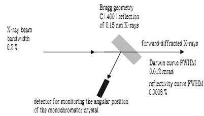
Figure 4: X-ray optics for compact crystal monochromator (see references in [1]) for a hard X-ray self-seeding setup.
