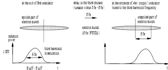
Figure 8: Principle of the fresh bunch technique for the high power mode of operation in the photon energy range between 3 keV and 5 keV. The third magnetic chicane smears out the electron microbunching and delays the electron bunch with respect to the radiation pulse. The unspoiled part of electron bunch is seeded by a GW level monochromatic pulse at third harmonic frequency. Tunability of the output pulse duration can be easily obtained by tuning the magnetic delay of the third chicane.
