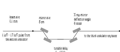
Figure 3: X-ray optical system for delaying the soft X-ray pulse with respect to the electron bunch. The X-ray optical system can be installed within the second magnetic chicane of the fresh bunch setup.
