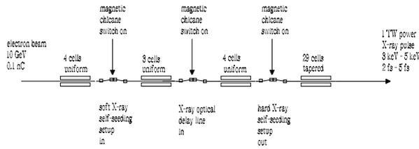
Figure 6: Design of the undulator system for 1 TW power mode of operation in the 3 keV - 5 keV photon energy range. The method exploits a combination of self-seeding scheme with grating monochromator, fresh bunch and undulator tapering techniques.
