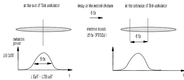
Figure 7: Principle of the fresh bunch technique for the high power mode of operation in the photon energy range between 3 keV and 5 keV. The second chicane smears out the electron microbunching and delays the monochromatic soft X-ray pulse with respect to the electron bunch of 6 fs. In this way, half of the electron bunch is seeded and saturates in the third undulator.
