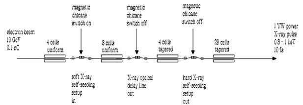
Figure 5: Design of the undulator system for 1 TW power mode of operation in the soft X-ray photon energy range. The method exploits a combination of self-seeding scheme with grating monochromator and an undulator tapering technique.
