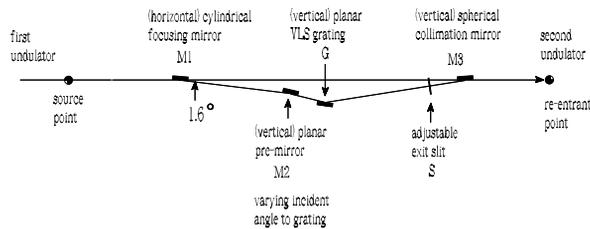
Figure 2: Optics for the compact grating monochromator originally proposed at SLAC (see references in[1]) for the soft X-ray self-seeding setup.
