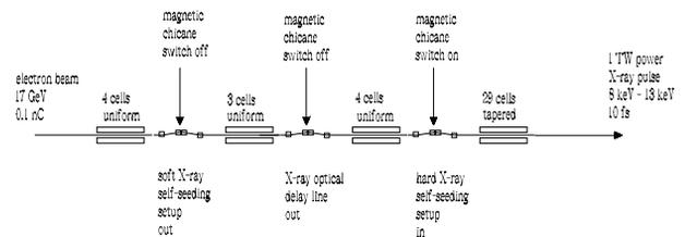
Figure 10: Design of the undulator system for 1 TW power mode of operation in the 8 keV - 13 keV photon energy range. The method exploits a self-seeding scheme with crystal monochromator.
