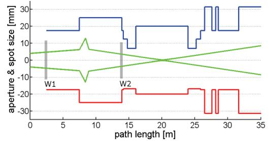
Figure 5: Vertical (blue) and horizontal (red) apertures of the laser path from BL3 to BL4, starting from the THG unit. The green curves denote the spot size ( $2\sigma$  radius) of the laser pulses, which pass through two vacuum windows (W1, W2) before entering the undulator.
