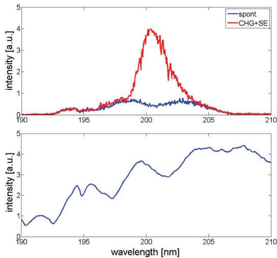
Figure 7: Spectrum of the spontaneous emission (blue) and coherent radiation (red) around 200 nm in air with a laser and modulator wavelength of 400 nm and the radiator tuned to the second harmonic. The top graph was acquired with a scanning PMT spectrometer and additional bandpass filters. The bottom graph shows only the spontaneous emission acquired with a CCD spectrometer without bandpass filters.
