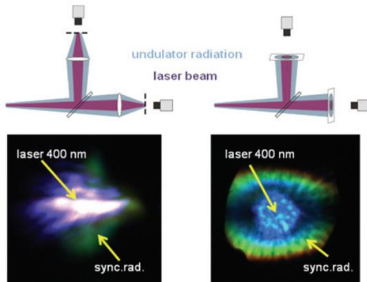
Figure 6: Transverse laser-electron overlap observed in the undulator (left) and on downstream screens (right).
