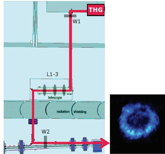
Figure 4: Sketch of the seed beamline BL3 (left). The laser pulses from the THG unit pass through two vacuum windows (W1, W2) and three lenses (L1-3) before entering the undulator, which leads to a donut-shaped laser profile (right).
