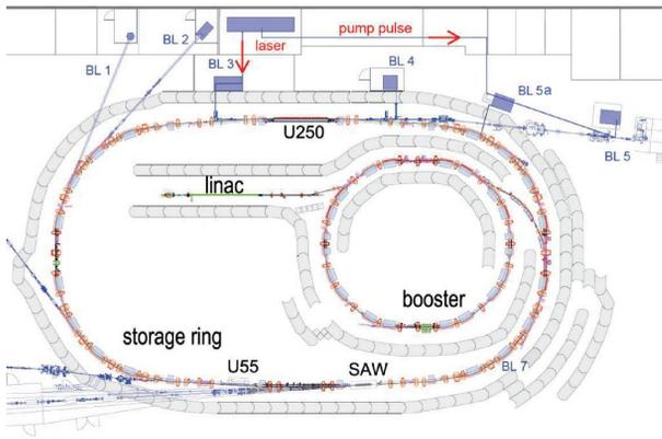
Figure 2: Overview of the DELTA accelerator complex.
