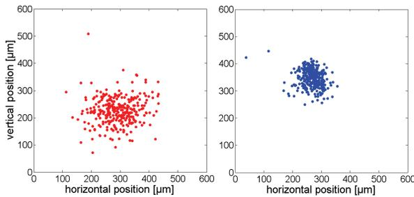
Figure 3: Position of the laser spot at the waist before (left) and after (right) covering the laser path on the optical table.
