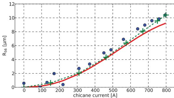
Figure 8: Dispersive strength  $R_{56}$  of the U250 chicane, determined by simulation (red curve), by field measurements (green dots), and by measured spectra of the optical klystron with both undulator parts tuned to 200 nm (blue dots).
