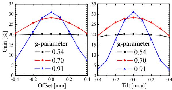
Figure 4: Effect of cavity misalignment under the condition of different g-parameters at 5.8 μm.
