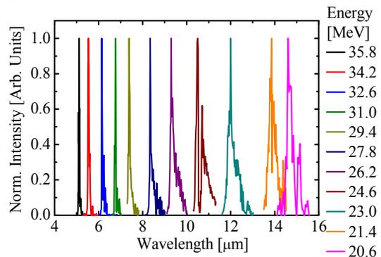
Figure 7: Spectrum of KU-FEL with various electron beam energy.
