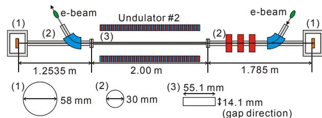
Figure 3: Geometry of the undulator and cavity mirrors.
