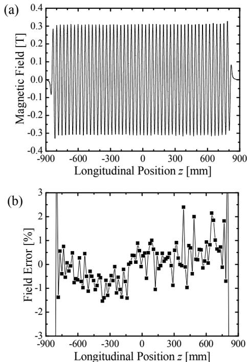
Figure 2: Measured magnetic field (a) and field error (b) of undulator #2 at the undulator gap of 20 mm.
