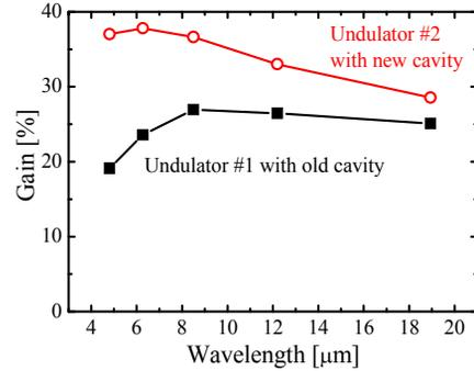
Figure 6: Net gain of undulator #2 with new optical cavity and undulator #1 with old optical cavity.
