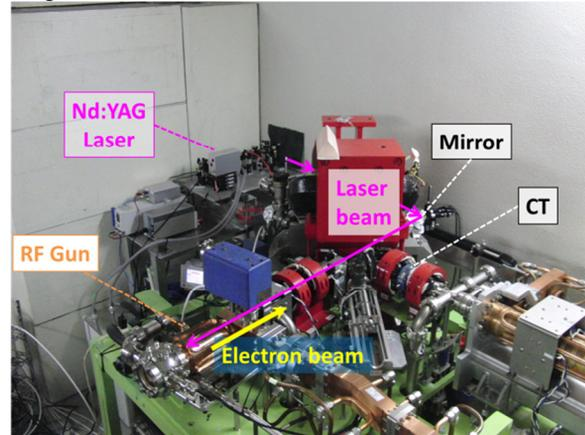
Figure 6: Set up for laser irradiation to thermionic and photo multiple-cathode.
