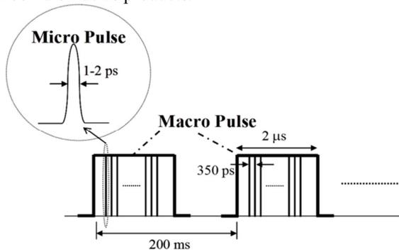
Figure 5: Pulse time structure of MIR-FEL output.
