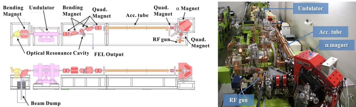
Figure 2: Schematic layout and Photograph of MIR-FEL.
