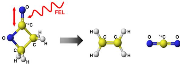
Figure 4: IRMPD of  $\beta$ -propiolactone gives ethylene and carbon dioxide as products.
