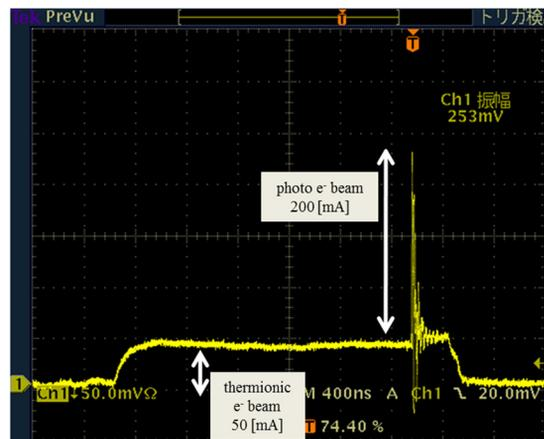
Figure 7: Thermionic and photo electron beam waveform measured by Current Transformer.
