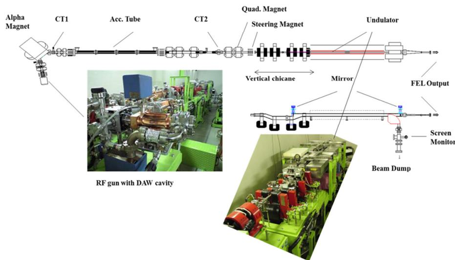
Figure 3: Schematic layout and Photograph of FIR-FEL.
