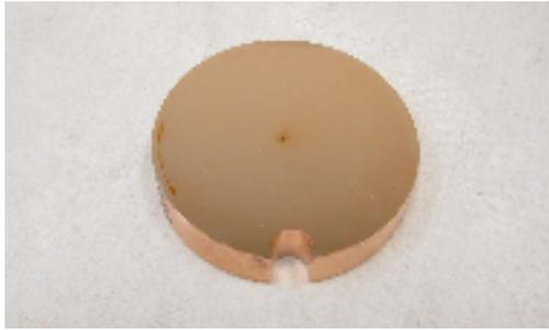
Figure 2: Damaged downstream mirror.
