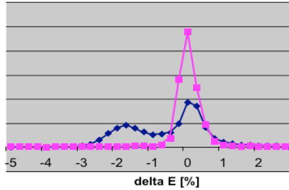
Figure 4: Electron beam energy spectrum, with (blue) and without (magenta) lasing.
