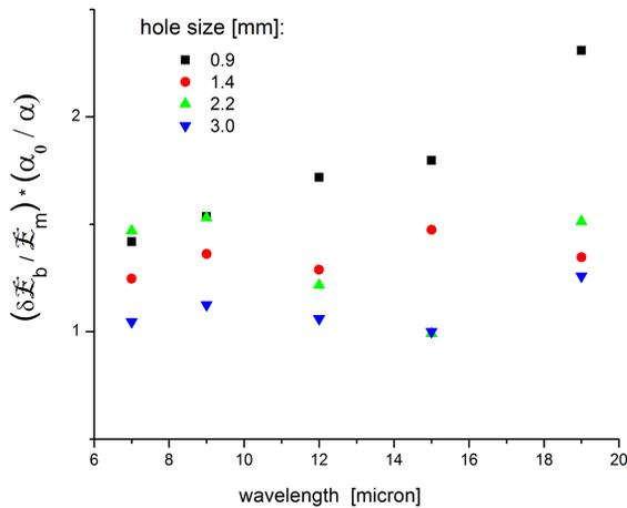
Figure 8: Ratio between extracted and optical energy at diagnostic station, corrected for transport loss.
