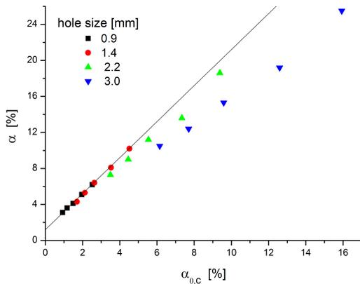
Figure 3: Roundtrip loss versus computed out-coupling, corrected for the damaged mirror. The drawn line has a slope of 2 and an offset of 1.2[%].
