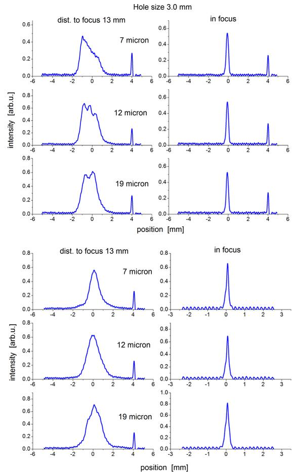
Figure 10: Spatial beam profiles measured in a user station, using a 150 mm parabolic mirror. Top 3 panels: hole size 3.0 mm, left: 13 mm from the focus, right: in the focus for 7 (top trace), 12 (middle) and 19 (bottom)  $\mu\text{m}$  respectively. Lower three panels: the same for the 1.4 mm hole size.
