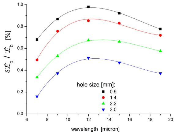
Figure 5: Relative energy extracted from the electron beam as a function of wavelength for three hole sizes.
