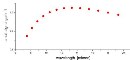
Figure 6: Typical computed small-signal gain.
