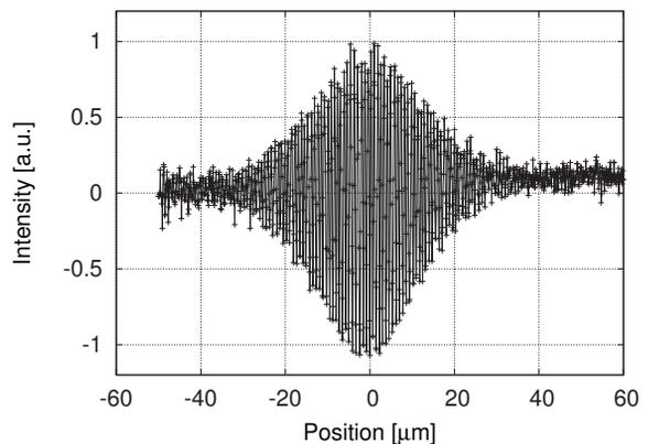
Figure 4: Autocorrelation trace in the superimpose mode.
