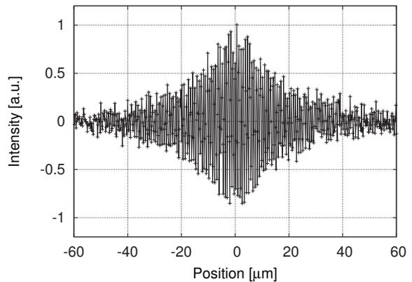
Figure 3: Autocorrelation trace in the burst mode.
