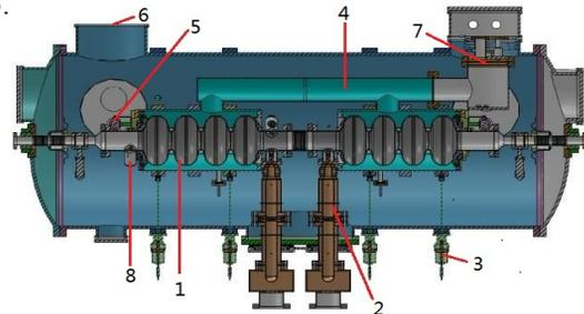
Figure 5: The superconducting module. 1 – 4cell cavity , 2 – microwave coupler , 3 – knighthead, 4 – 2K shield, 5 – tuning system, 6 – inlet port of liquid nitrogen, 7 – inlet port of liquid helium, 8 – HOM coupler.
