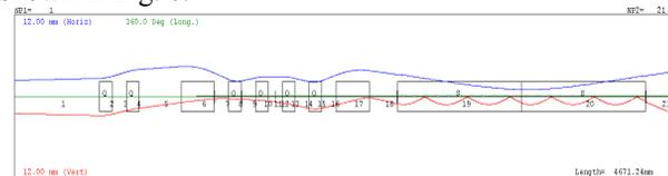
Figure 6: Electron beam envelope in the transport system.
