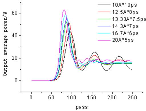
Figure 2: Output average power as a function of electron current.
