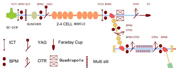
Figure 7: Schematic of beam diagnostics.
