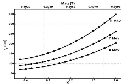
Figure 8: Wavelength ranges as a function of wiggler parameter K for the indicated values of the electron kinetic energy.
