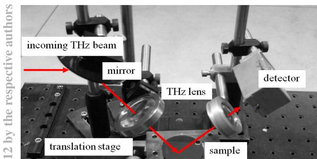
Figure 7: the reflection mode THz imaging setup.
