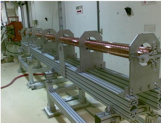
Figure 1: The rf linac for the NSRRC thermionic rf gun injector.
