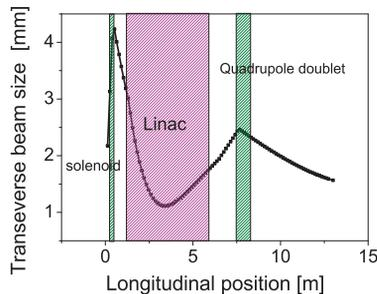
Figure 3: Transverse beam size tracked from cathode through the linac to the end of the chicane (calculated with ASTRA 3D). Chicane magnets are switched off here (bunch charge 3 nC, laser pulse length 4 ps).
