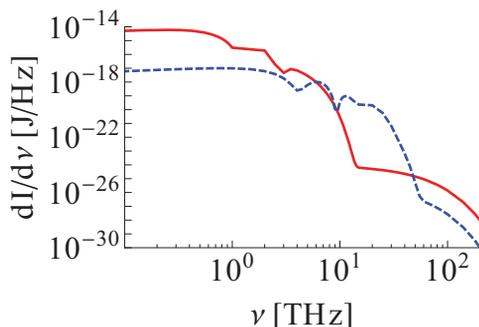
Figure 8: CSR spectrum for the 3 nC (continuous) and 100 pC (dashed) bunches.
