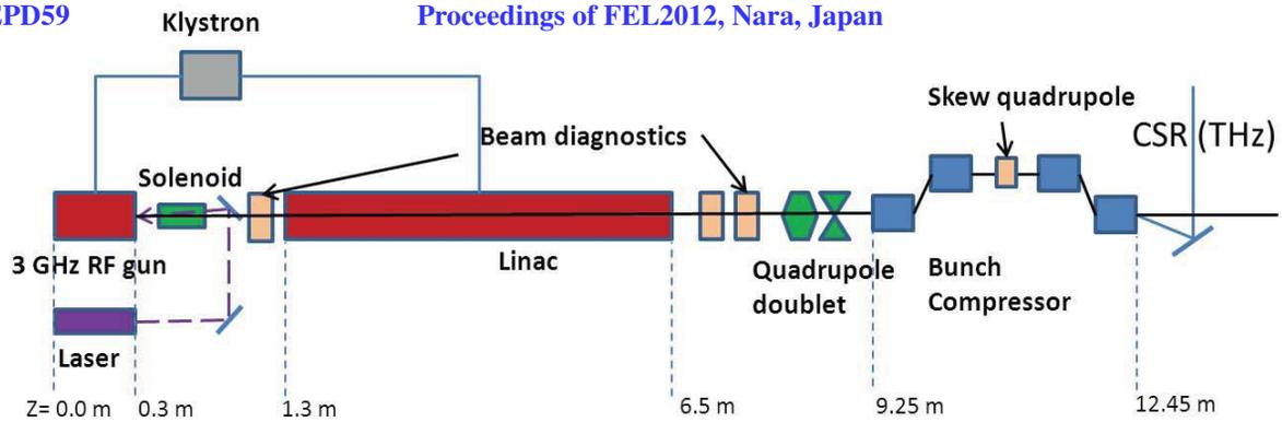
Figure 1: Schematic FLUTE layout (not to scale).
