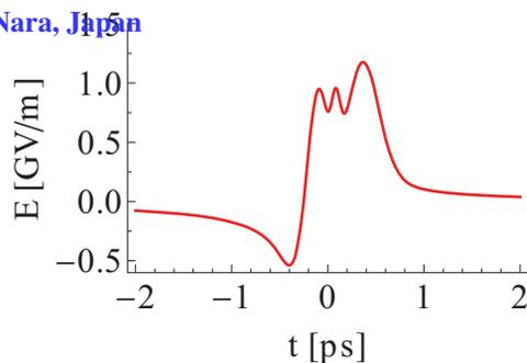
Figure 9: The focused electric field pulse calculated from the 3 nC bunch charge.
