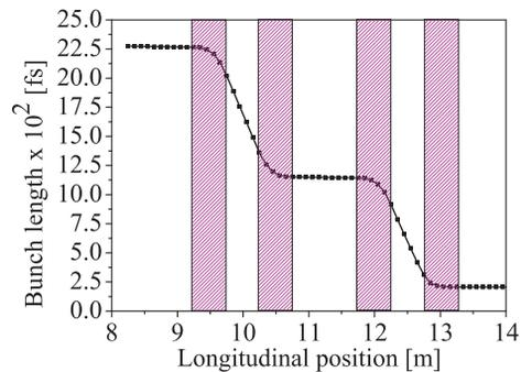
Figure 4: The development of the bunch length tracked through the compressor using ASTRA 3D routines. The shaded parts symbolize the position of the magnets (here 50 cm long).
