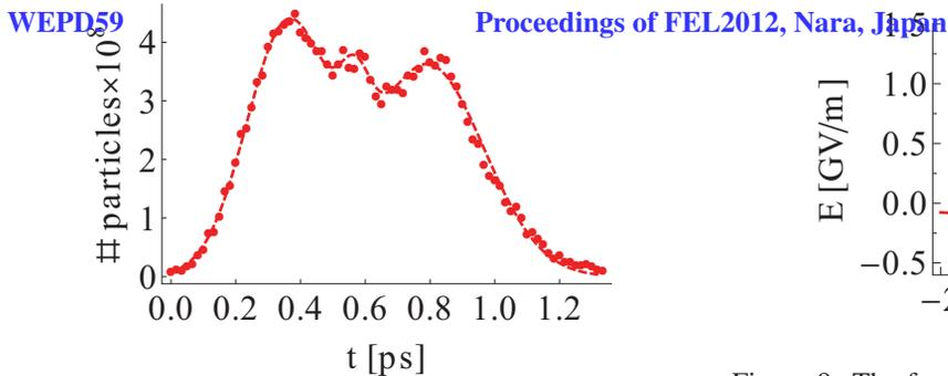
Figure 7: Longitudinal charge profile for a 3 nC bunch at the exit of the fourth chicane magnet. The dashed curve is a Gaussian fit of the data.
