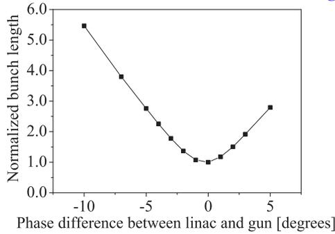
Figure 5: Compressed bunch length as a function of the phase difference between gun and linac cavities calculated with 1D CSRtrack (3 nC charge, 4 ps laser pulse length).
