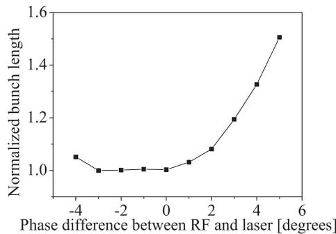
Figure 6: Bunch length as a function of the phase difference between laser pulses and RF signal, calculated with 1D CSRtrack (3 nC, 4 ps laser pulse length).
