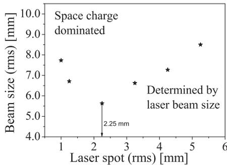
Figure 2: Optimized electron vs laser spot size at the exit of the solenoid after the gun as calculated with ASTRA 3D. For laser spot sizes smaller than 2.25 mm the beam size is increased by space charge effects, for larger spot sizes the beam size is dominated by the laser spot size (bunch charge 3 nC, laser pulse length 4 ps).
