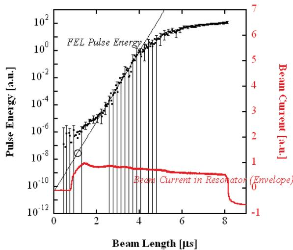
Figure 2: Measured energy development of FEL macropulse.
