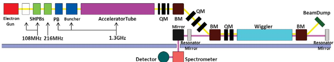
Figure 1: Diagram of L-band linac and THz-FEL.
