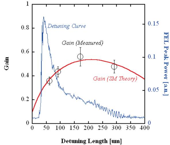
Figure 5: Small signal gain vs detuning length and comparison to Super-Mode theory.
