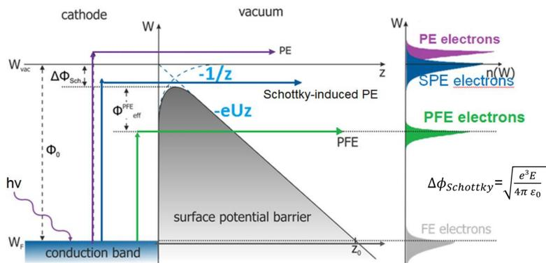
Schematic of the FE, PE, SPE and PFE processes with energy distributions of the emitted electrons.
