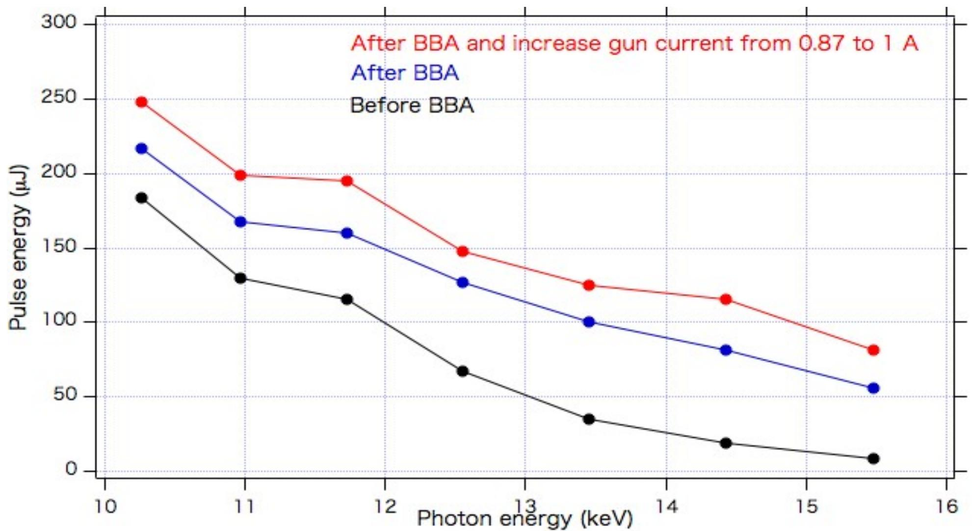
Beam energy at 7.8 GeV, K-value scanned from 2.1 to 1.5.
