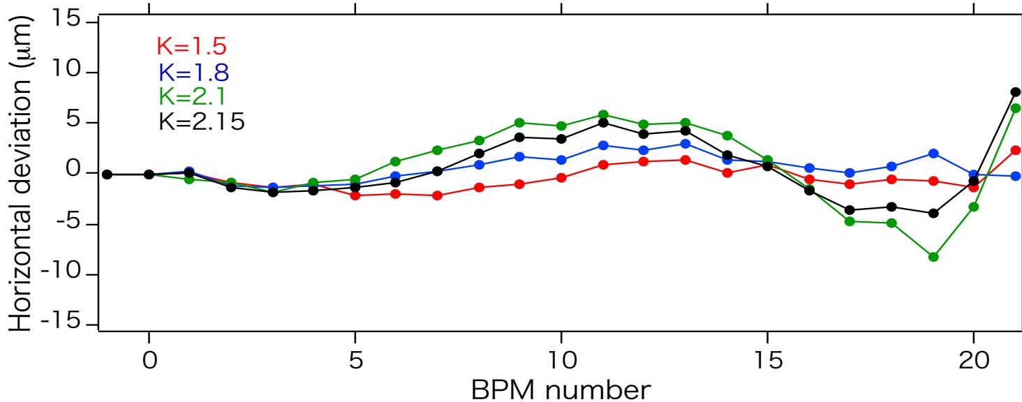
Orbit deviation with respect to 10 mm gap reference.
