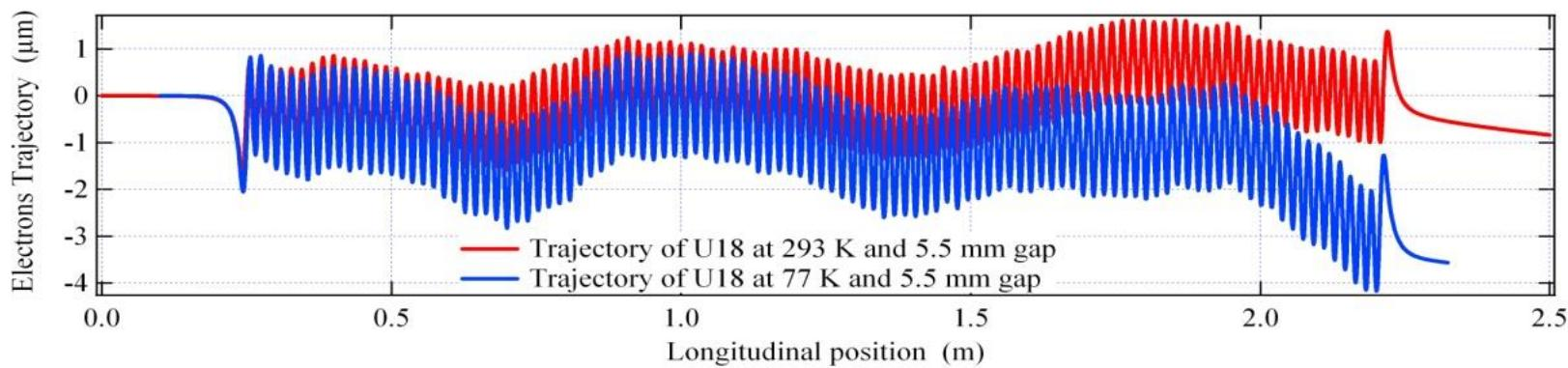
Correction of the electron trajectory angle (9 μm) at 77 K
