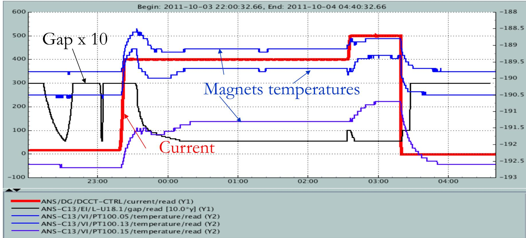
Thermal gradient on the magnetic system  $< 1.5 \text{ K/m}$
