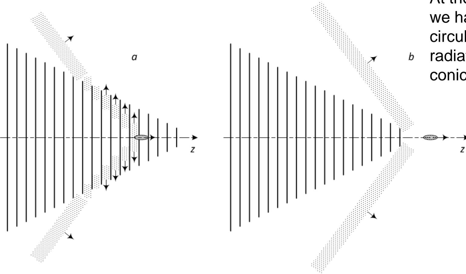
At the cone outer surface we have synchronized circular radiators. Their radiation field forms the conical wave (see Fig. 1b).
