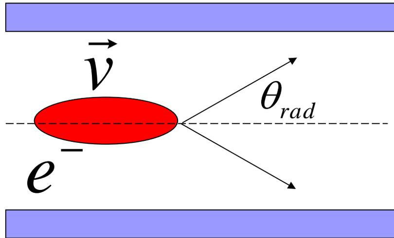
The diffraction angle of radiation is inversely proportional to the electron beam energy.
