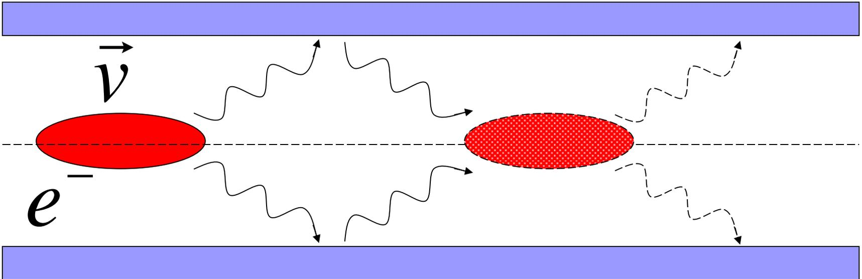
The tube's length must be on the order of the undulator gain length
