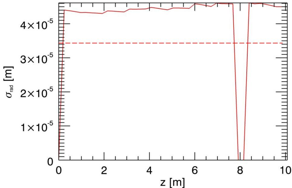
Simulation over 10 meters without the tube. Radiation rapidly grows and without restraint.
