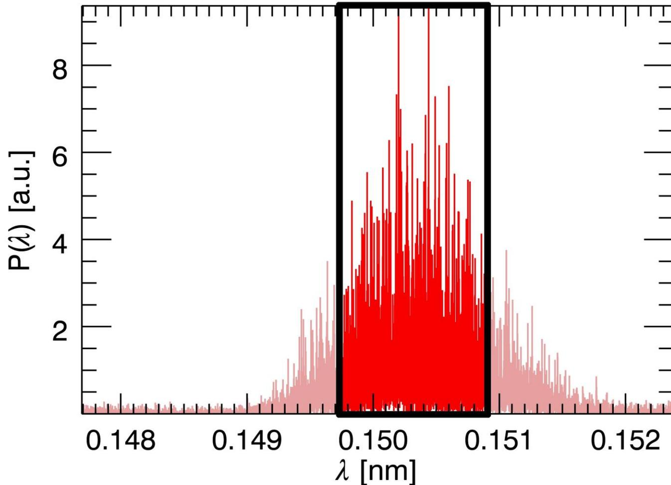
We use a simple hard-edge frequency filter model
