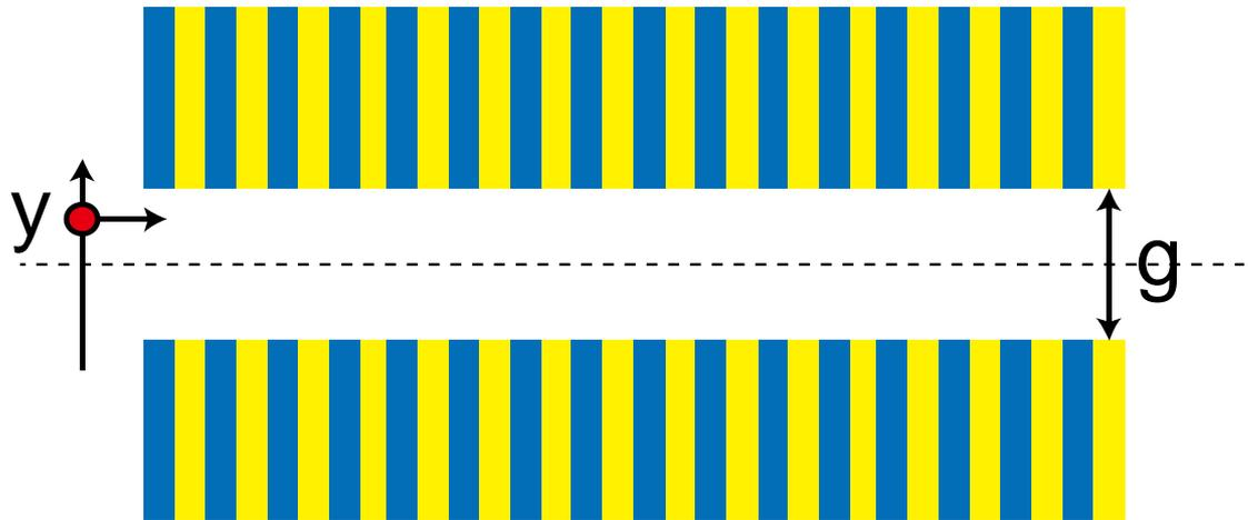
Both the undulator gap and height should be aligned for precise K value tuning!
