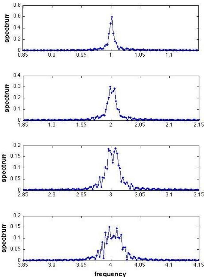
After the chicane beam compression varies along the bunch due to the nonlinear chirp
