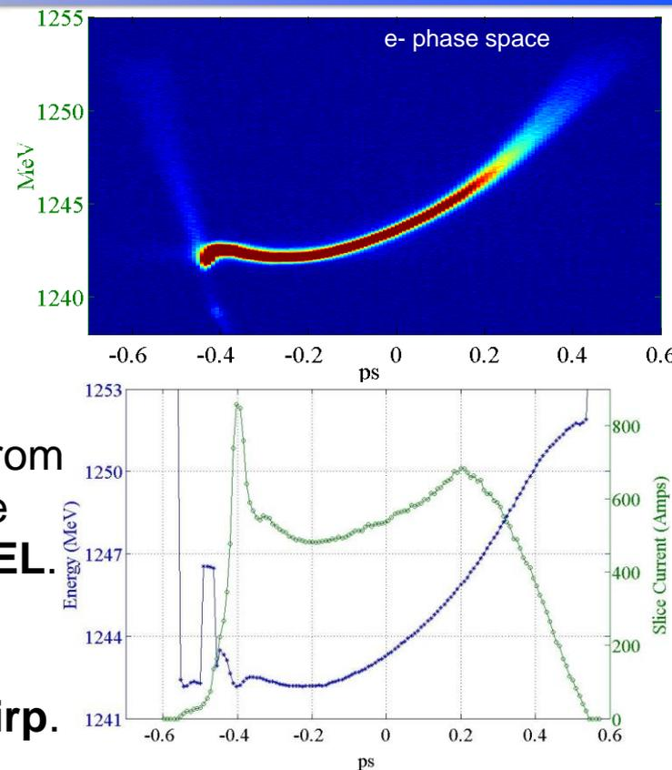
By measuring the **FEL spectra** as a function of the seed laser delay we can look at the **effects** of the **e- beam phase space** into the FEL.
