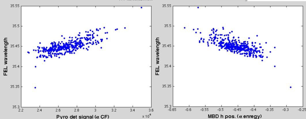
Measurements during users operations indicate that wavelength fluctuations are strongly correlated with the beam properties fluctuations in BC1 (compression) and in main beam dump (energy) .
