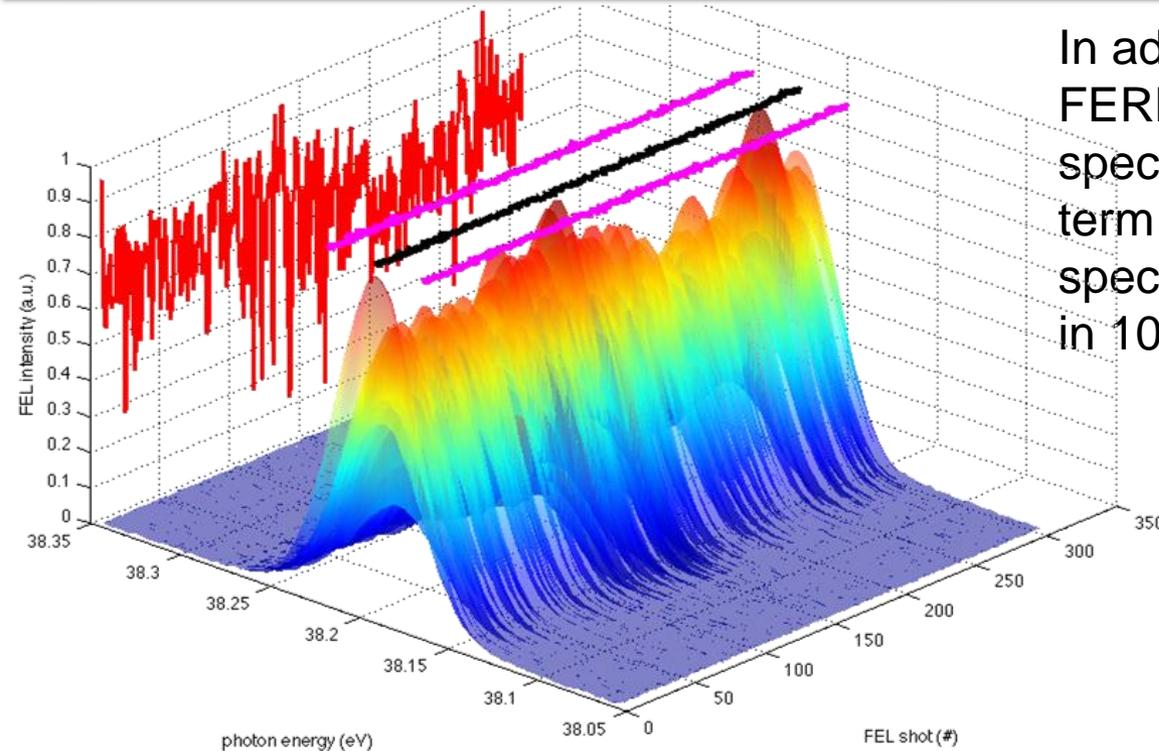
Reported data refer to an electron beam of 350pC at 1.24GeV compressed about a factor 3. The 6 radiators are tuned to 32.5nm.
