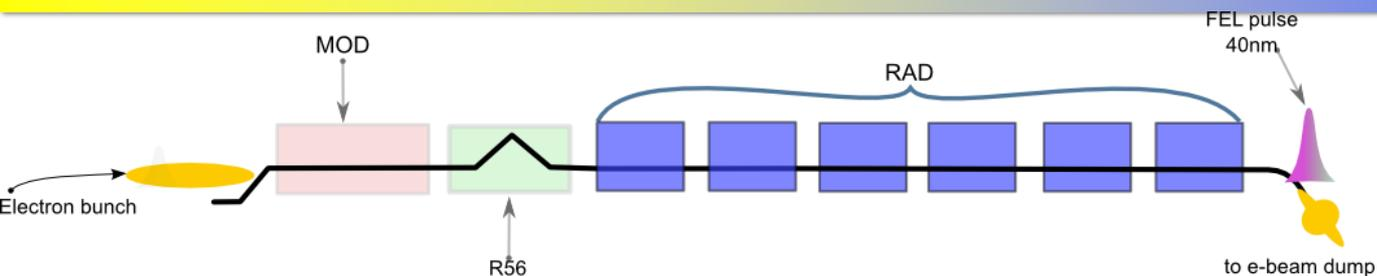
Highly compressed beam with 6 undulators tuned at ~40nm in circular polarization
