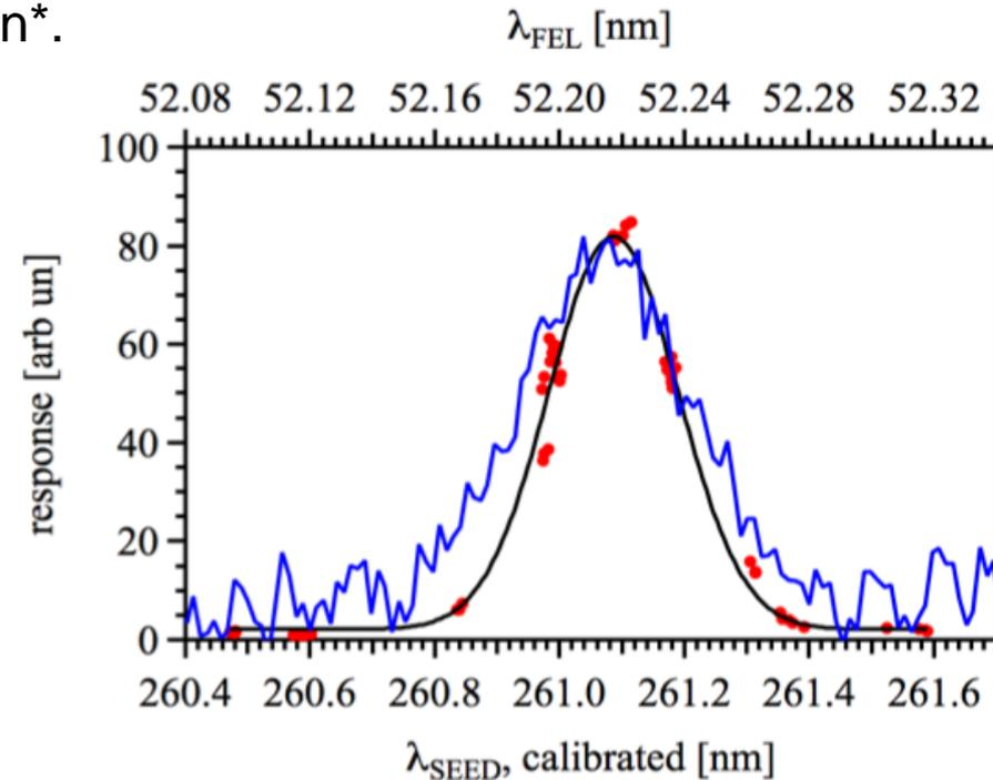
**Figure 10.** Reconstructed He absorption profile (red dots: PMT response vs calibrated wavelength; black line: gaussian fit), and comparison with Padres spectrometer trace (blue line). Note  $\lambda_{FEL} = \lambda_{SEED}/5$ .
