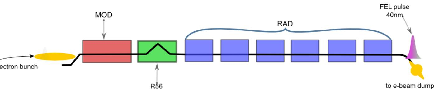
SASE signal is strongly enhanced by using the optical klystron configuration, with modulator tuned at the same wavelength and small dispersion in R56.
