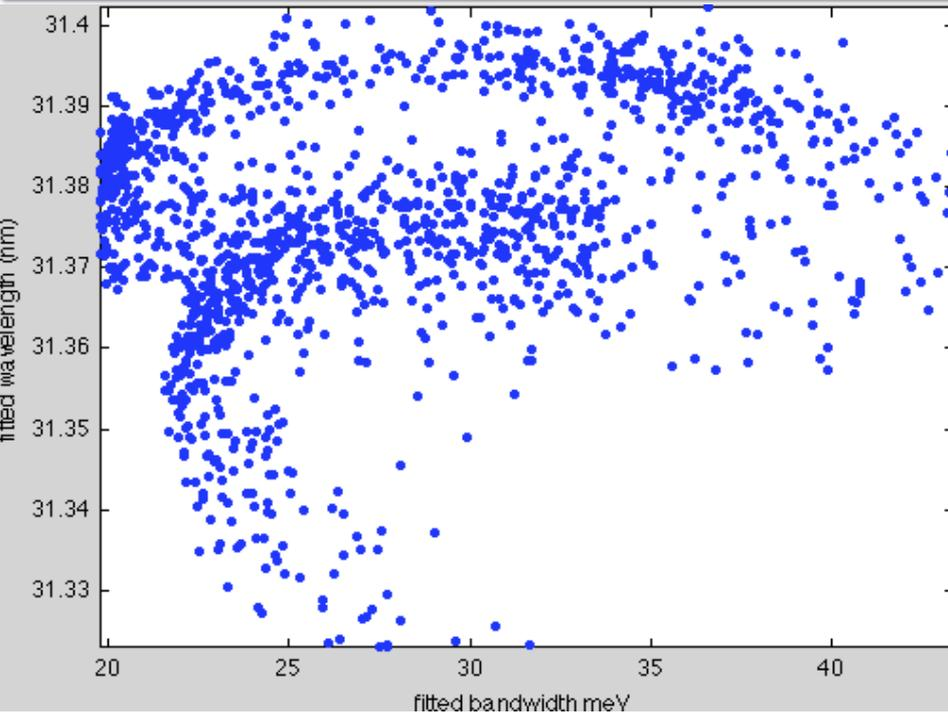
By plotting the **central wavelength** as a function of the **bandwidth** we find strong **correlations**. This suggests that **fluctuations** are related to electron **beam phase space** and **timing jitter**.
