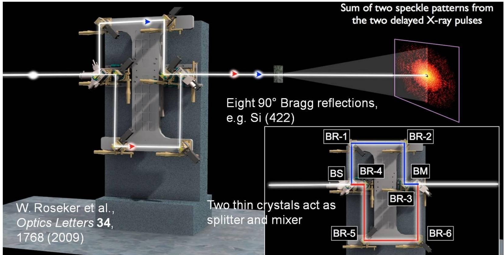
90° diffraction angle gives fixed energy: 8.4 keV for Si (511), 7.9 keV for Si (422)
