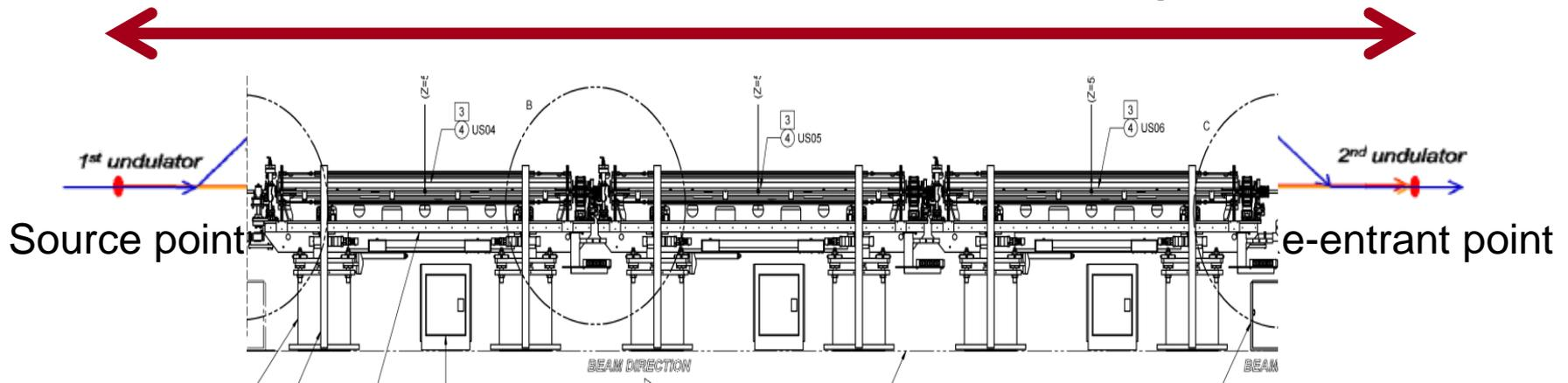
Figure 1: Schematics of the optics for soft X-ray self-seeding the LCLS-II.
