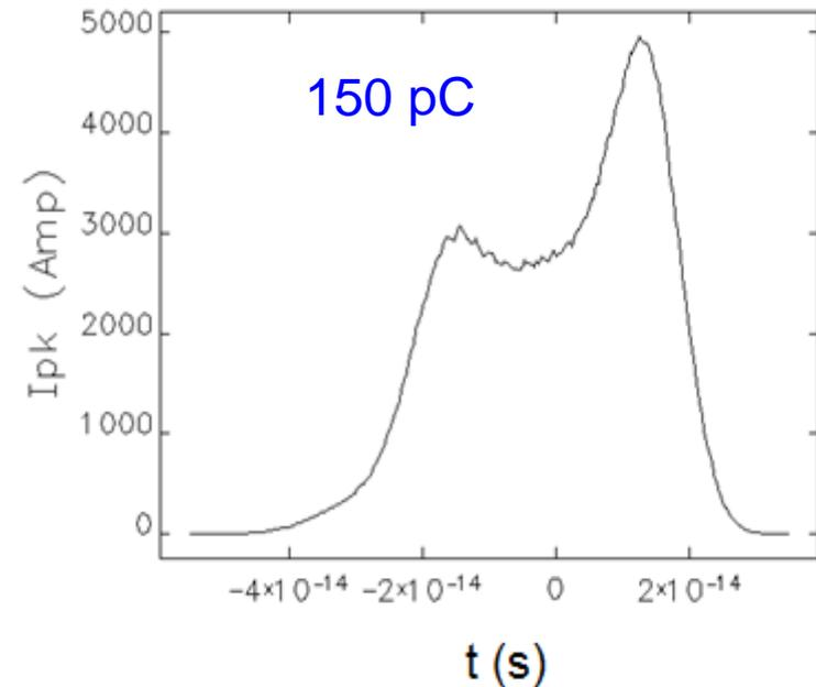
Double-horn profile of the electron bunch compressed to 3 kA peak current in the central part.
