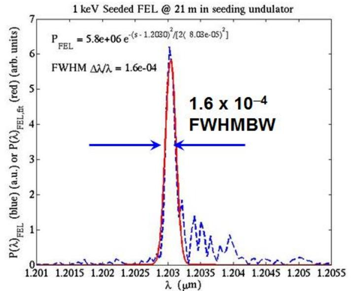
Seeded FEL spectrum at 21 m in the SASE undulator.
