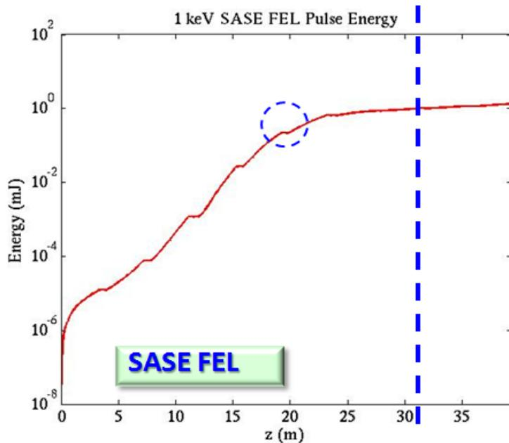
SASE FEL gain curve. The dashed vertical line stands for the end of U8; the dashed circle stands for the operation point.
