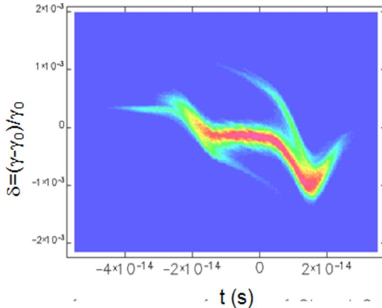
Longitudinal phase space of the electron bunch at the entrance of undulator system.
