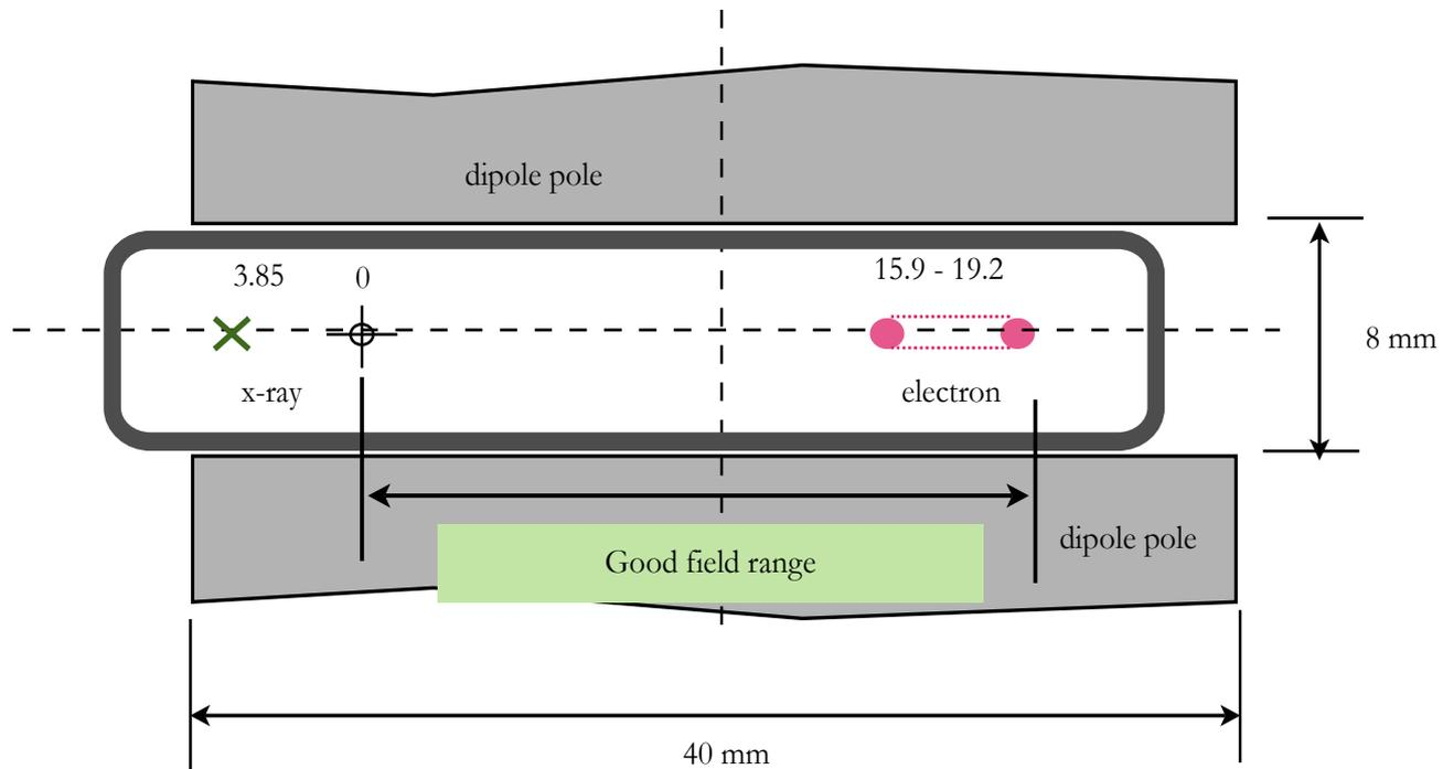
Beam paths with horizontal displacements noted for the electron and X-ray beams are shown for the 1 keV case.
