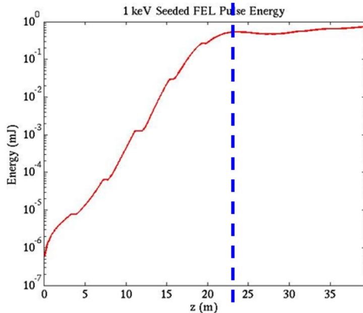
Seeded FEL gain curve. The dashed vertical line stands for the end of U15.
