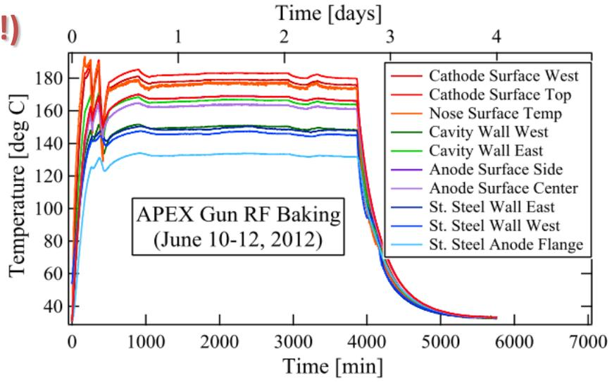
Only 1 NEG out of 20 activated after the 2.5 days RF baking.
