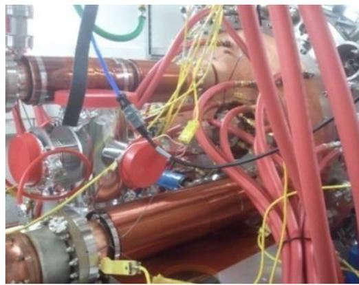
RF Feeder Ant-Multipacting Setup
