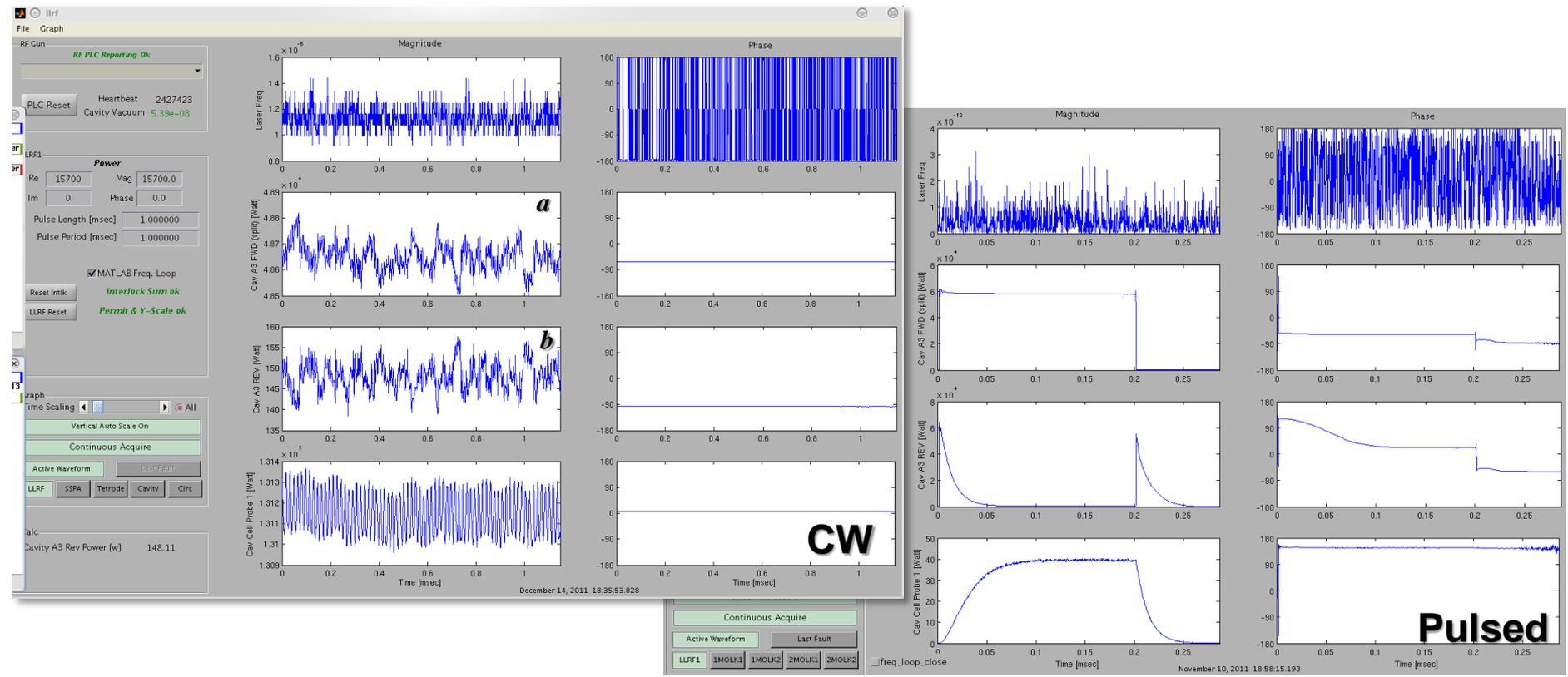
On Dec. 15, 2011 after < 120 integrated hours of conditioning, more than 12,5 hours run without faults were achieved in CW mode at nominal power (100 kW). Results reconfirmed the day after (> 24 hours no fault).
