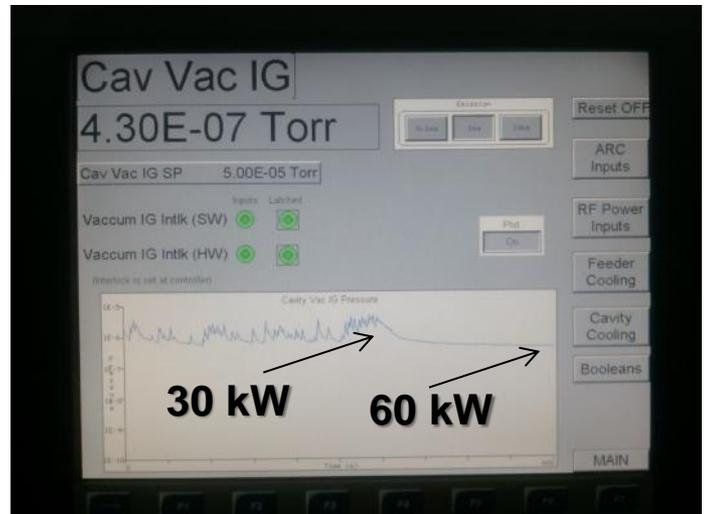
The two Toshiba RF windows were conditioned at the full power of 60 kW (in less than twenty hours). **Good system cross-check.**
