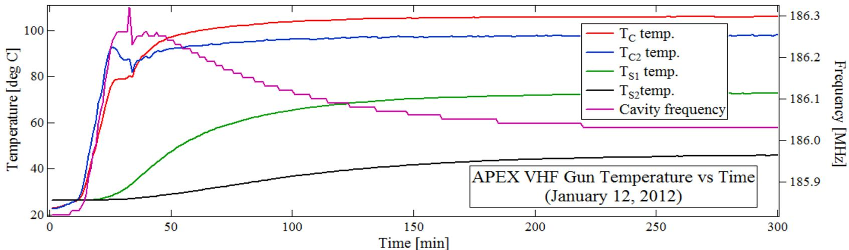
We have two “regimes”: cold cavity in the first ~ 30 min where the copper is going to temperature; warm when the copper temperature stabilizes.
