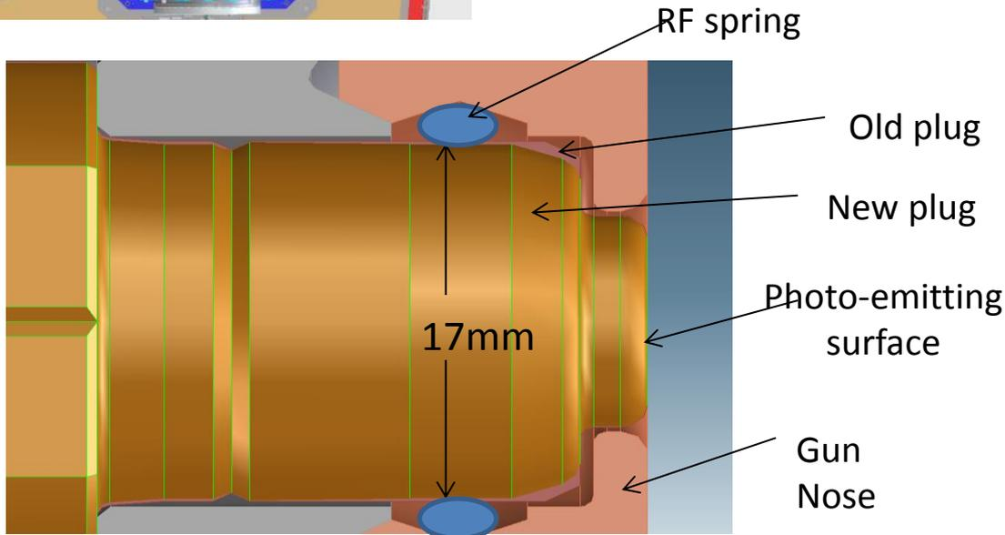
**Any photocathode deposited on a same geometry plug can be potentially tested at the VHF gun**
