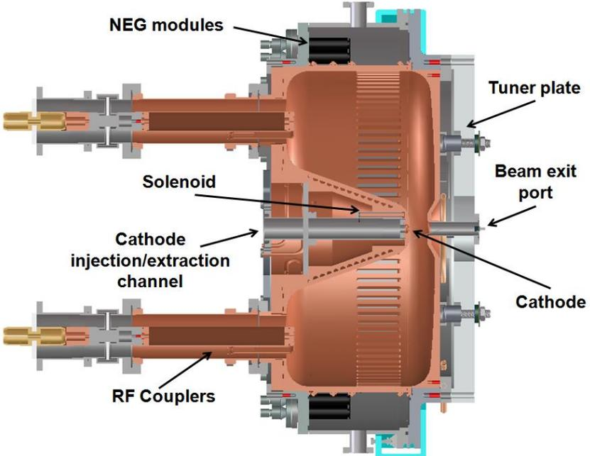
**Baking the gun with no water cooling (!) and 2-4 kW average RF power.**
