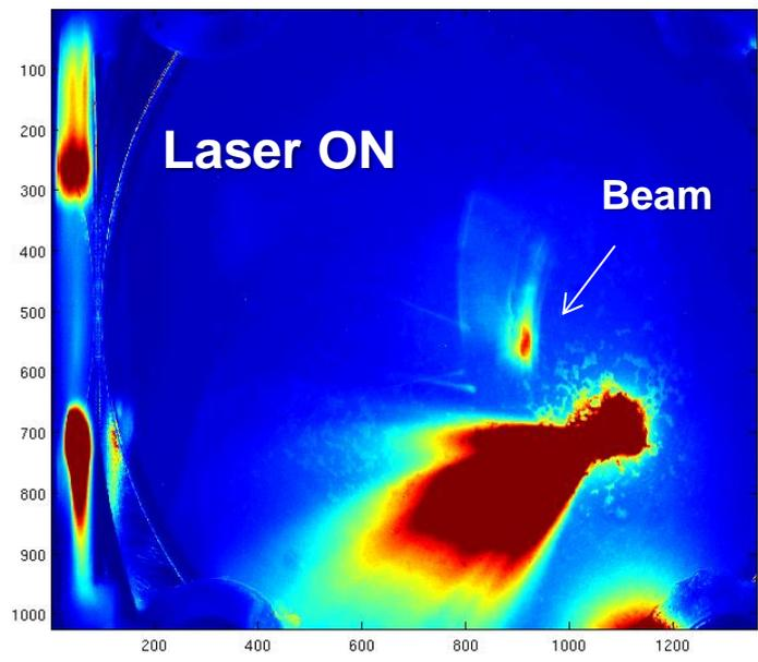
**Laser average power at the cathode: ~ 30 mW at ~ 266 nm.**
