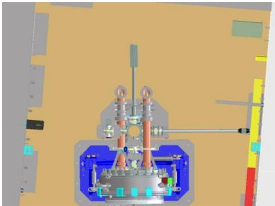
Adapted version of the INFN/PITZ/DESY load-lock system
