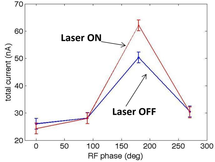
**Laser average power at the cathode: ~ 30 mW at ~ 266 nm.**
