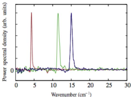
Typical emission spectra induced by the shaped laser pulses.
