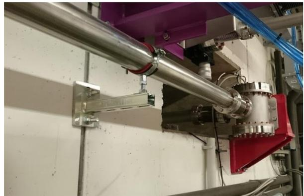
Figure 1: Vacuum chamber located close to the electron gun in the injector hall (red mount). The laser is redirected from the vertical shaft downstream the tunnel wall.
