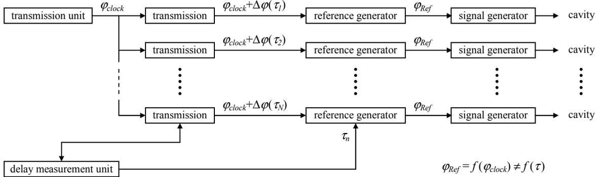
Figure 2: Basic principle of the cavity synchronisation.
