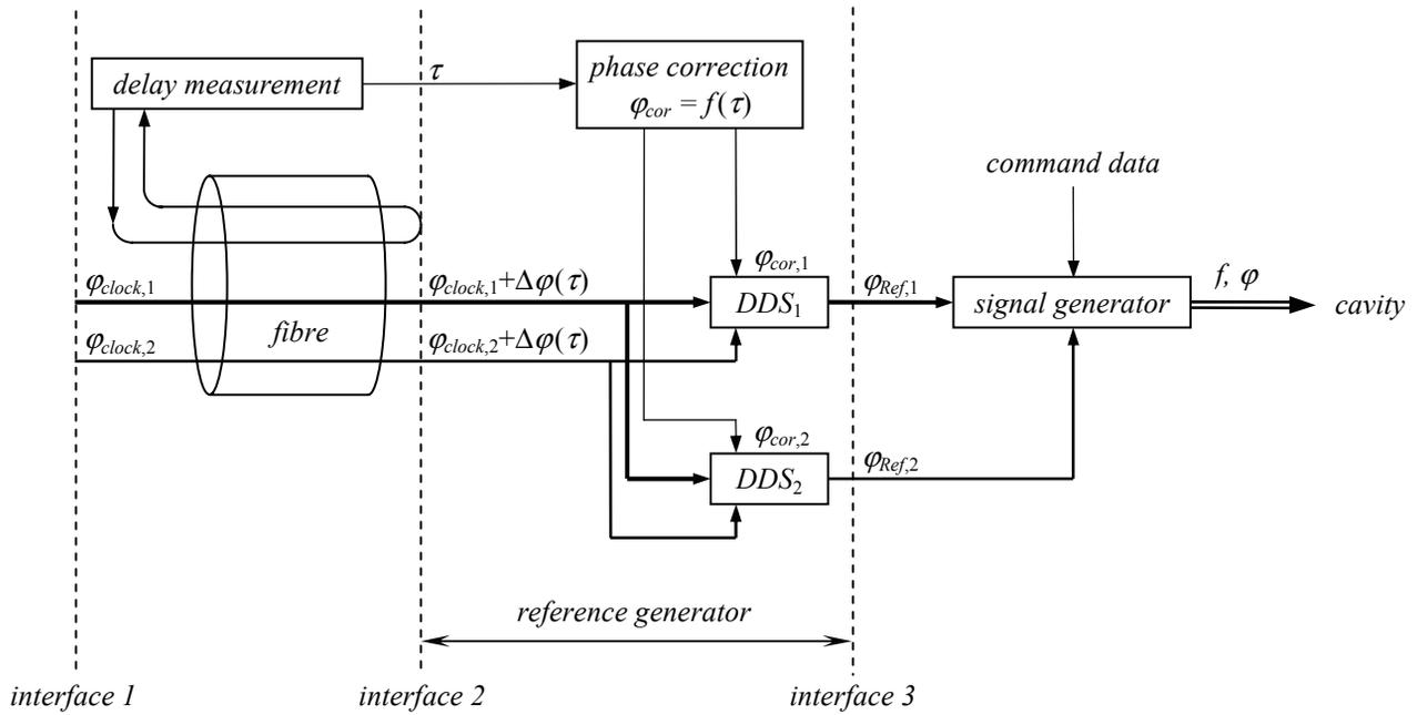
Figure 4: Generation of the reference signals.
