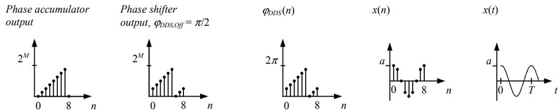
Figure 3: Direct digital synthesis principle.
