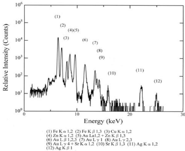
Figure 6: PIXE spectrum of the gilded frame of art works including one from Florence.
