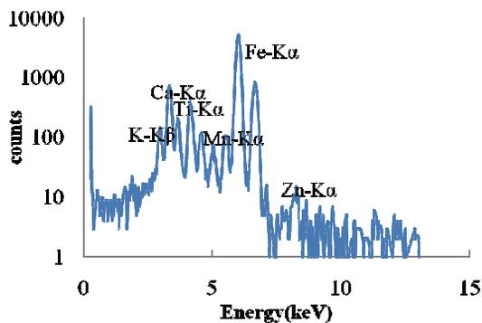
Figure 4: PIXE spectrum of pond sediment. This is that of “Sanshiro-ike” pond in the University of Tokyo.
