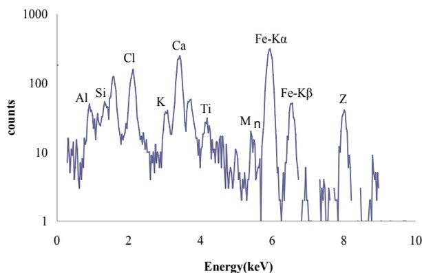
Figure 5: PIXE spectrum of SPM corrected in the campus of University of Tokyo.
