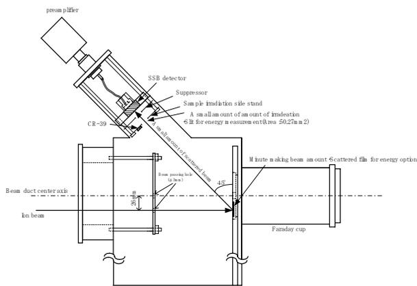
Figure 8: Schematic drawing of new irradiation system.
