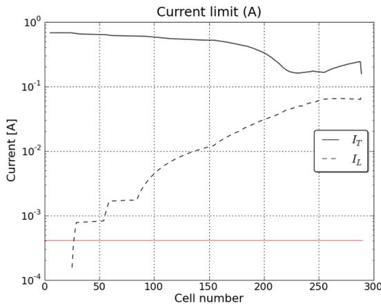
Figure 1: Current limit with smooth approximation line ( $I_T$  is transverse current limit and dashed line;  $I_L$  is longitudinal current limit)
