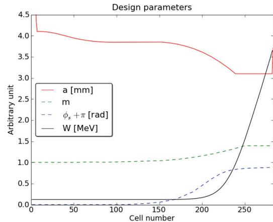
Figure 2: Main design parameters of RFQ consisting of a(aperture), m(modulation), phi(synchronous phase) and W(kinetic energy of synchronous particle)
