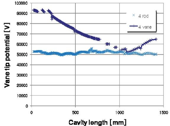
Figure 6:  $V_0$  distributions of two RFQ structure
