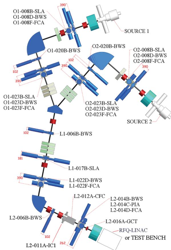
Figure 1: LEBT line layout. Sketch of magnets and beam diagnostics monitors, from the sources to the test bench installed at the end of the LEBT line, during LEBT commissioning, in place of the RFQ. Legend: SLA= Slit monitor, FCA= Faraday Cup monitor, BWS= Wire Scanner, CFC= Chopper Faraday Cup monitor, GCT= AC- Current Transformer, PIA= Wires Harp, IC1= Chopper magnet.
