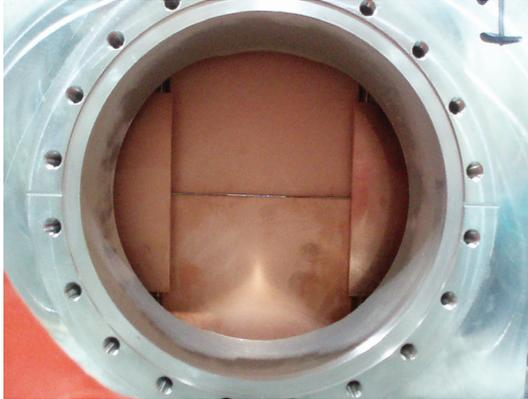
Figure 6: The four Copper plates, making one Slit monitor, installed on their tank. Left and right plates are positioned at beam border; top and bottom plates are making a very thin slit at about tank center.
