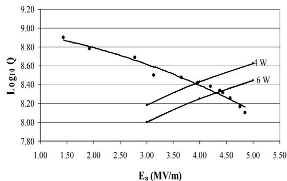
Figure 2: Offline performance of one of the indigenously built QWRs at 4.5 K.
