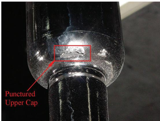
Figure 4: Punctured upper cap on the central conductor of the coaxial line.
