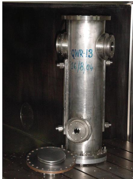
Figure 1: One of the indigenously built niobium quarter wave resonators along with the slow tuner bellows.
