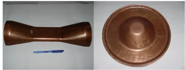
Figure 8: (a) Left – Half Spoke formed in copper and after machining the edges and ends. (b) Right – End Wall formed in copper. The edge has not been machined.
