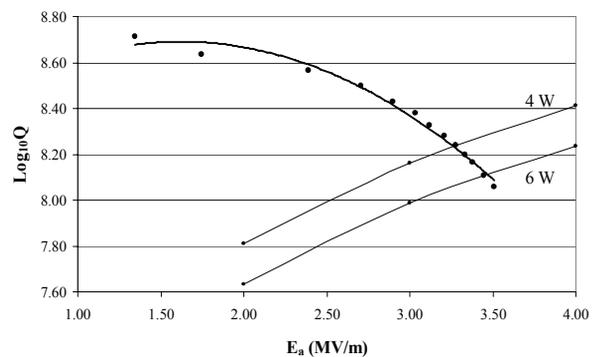
Figure 6: Offline performance of one of the repaired resonator QWR-6 at 4.5 K.
