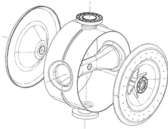
Figure 7: 325 MHz,  $\beta=0.22$  Single Spoke Resonator. The outer shell diameter is 498 mm.
