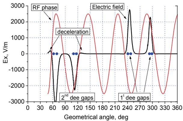
Figure 8: The RF phase and azimuth component of electric field acted on  $^{48}\text{Ca}^{5+}$  central ion.
