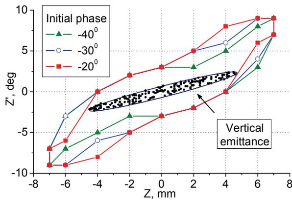
Figure 4: “A” operation mode. The cyclotron vertical acceptance and  $^{48}\text{Ca}^{5+}$  ions beam emittance.
