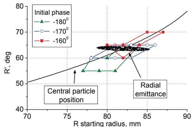
Figure 7: “C” operation mode. Radial acceptance and optimal position of the  $^{48}\text{Ca}^{5+}$  ion beam emittance.
