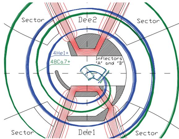
Figure 2: The first orbits of  $^4He^{1+}$  and  $^{48}Ca^{7+}$  ion beams at 2 and 3 RF harmonics respectively. In the figure “A” and “B” operation modes are combined.
