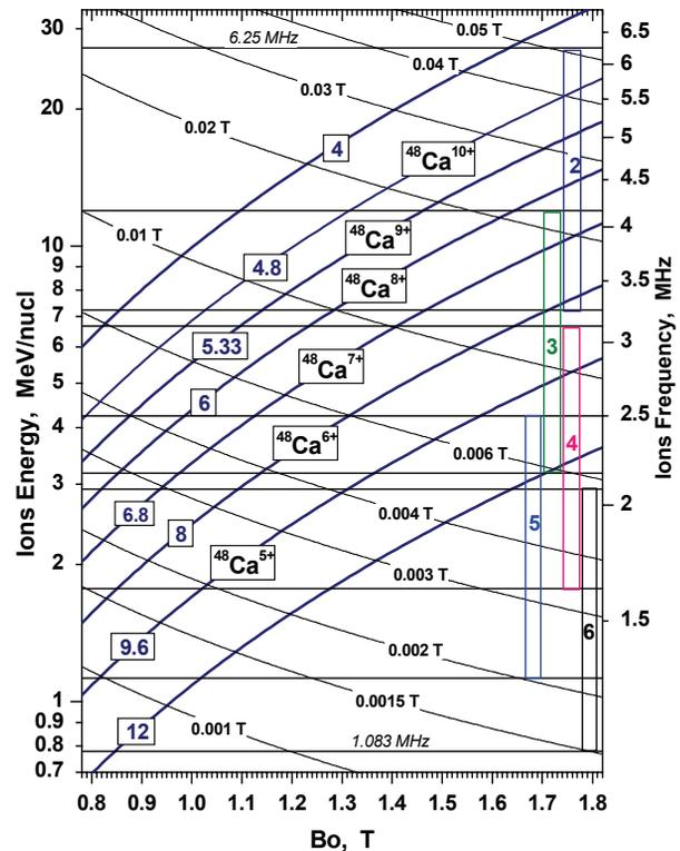
Figure 1: The working diagram of the U400R cyclotron.
