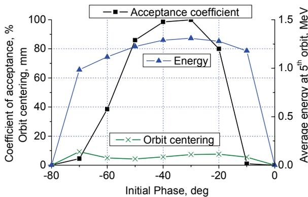
Figure 5: The efficiency, orbit centring and average energy of  $^{48}\text{Ca}^{5+}$  ion beam at the central region.
