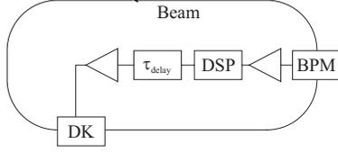
Figure 2: Layout of a classical transverse feedback system.
