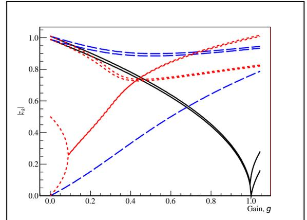
Figure 5: Dependences of damping rates  $|z_k|$  on gain  $g$  for the ideal TFS (solid curves), for the TFS with the notch filter (dashed curves) and for the TFS with the notch and all-pass filters (dotted curves), parameter  $a = -0.501$ ; shown is the case of the tune of  $Q = 6.73$  and an assumed instability rise time of  $\tau_{\text{inst}} = 100T_{\text{rev}}$ .
