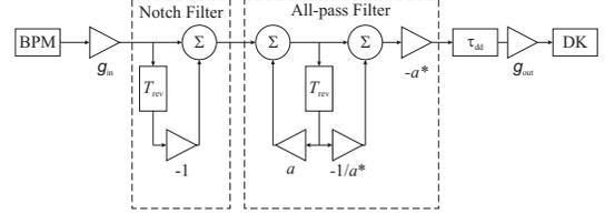
Figure 4: Block diagram of feedback loop with the notch and all-pass filters.
