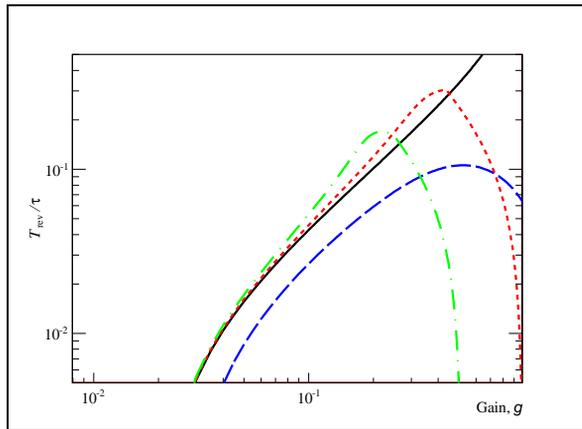
Figure 6: Dependences of overall damping rates  $T_{\text{rev}}/\tau$  on gain  $g$  for feedbacks: the ideal TFS (solid curve), with the notch filter (dashed curve), with the notch and all-pass filters for  $a = -0.501$  (dotted curve), with the notch and Hilbert filters for  $\Delta\varphi = -72.8^\circ$  (dash-dotted curve); shown is the case of the tune of  $Q = 6.73$  and an assumed instability rise time of  $\tau_{\text{inst}} = 100T_{\text{rev}}$ .
